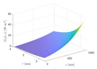
Fig. 9 Eqn (22) evaluated from  $R_i = 1.59$  mm to  $R_o = 3.87$  mm and z =0 to z = 0.94 m for  $\kappa_{\lambda} = 379 \text{ m}^{-1}$  and  $\Phi_{LDF} = 0.275 \text{ W}$ .
