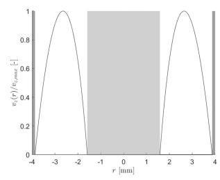
Fig. 8 Normalized axial velocity profile  $(v_z(r)/v_{z,max})$  as a function of radial position r for the constructed CAP-Flow system. The lightshaded area denotes the space occupied by the FEP tubing, while the dark-shaded area represents the external SS tubing.
