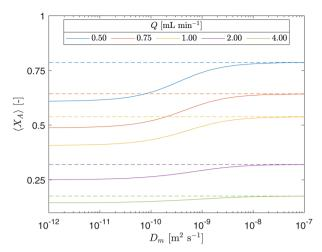
Fig. 12 Continuous lines: Effect of molecular diffusivity  $D_{\rm m}$  on fractional conversion  $(X_A)$  for a fixed photocatalyst concentration  $(C_{PC})$ of 70.0  $\times$  10<sup>-5</sup> equiv. while maintaining  $k \cdot \phi_{\lambda} = 0.0179 \text{ m}^3 \text{ einstein}^{-1}$ Dashed lines: Ideal plug flow model.
