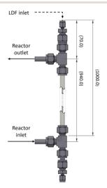
Fig. 3 Schematic representation of the CAP-Flow system; all dimensions are in millimeters.
