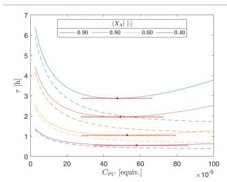
Fig. 14 Iso-conversion curves illustrating the relationship between mean residence times ( $\tau$ ) and photocatalyst concentrations ( $C_{PC}$ ). The continuous lines represent the solution of the partial differential equation (PDE) with a diffusivity of  $D_{\rm m}=10^{-10.2}~{\rm m}^2~{\rm s}^{-1}$ , while the dashed lines depict the ideal plug flow model solution. A red marker and horizontal dotted line indicate the minimum point for clarity.
