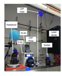
Fig. 4 (a) Experimental set-up in fume hood. (b) Process flow diagram.
