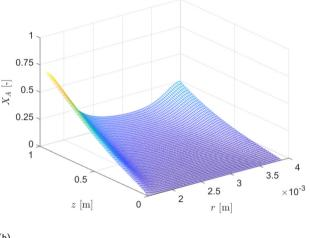
Fig. 11 PDE solution  $X_A(r, z)$  examples for  $C_{PC} = 20.0 \times 10^{-5}$  equiv. for two different flow rates. (a) Q = 0.5 mL min<sup>-1</sup>. (b) Q = 2 mL min<sup>-1</sup>
