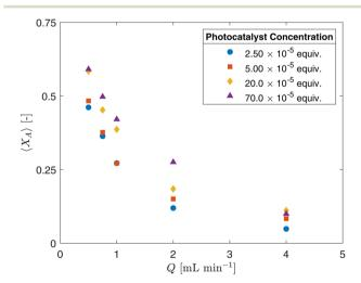
Fig. 6 Fractional conversion  $X_A$  as a function of flow rate Q for selected photocatalyst concentrations ( $C_{PC}$ ).
