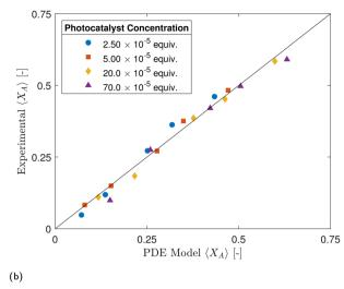
Fig. 10 (a) Fractional conversion  $(X_{\Delta})$  as a function of flow rate (Q) for different photocatalyst concentrations  $(C_{PC})$ . Markers represent experimental data, while the continuous lines represent values predicted by the PDE model. (b) Parity plot.
