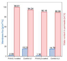
Fig. 12 Fluxes of membranes (left, blue dashed) and water content of the permeate (right, red) obtained during pervaporation coupled with esterification experiments (T = 95 °C, sweep gas p = 3/2 bar (feed/permeate)).
