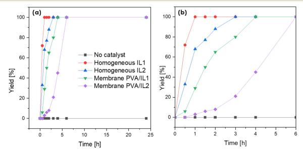
Fig. 9 Time evolution of esterification yield measured after batch esterification (T = 90 °C, under stirring) with no catalyst, catalyst added directly to the reaction flask and with PVA/IL-coated membranes (a) and magnification after cut-off at 6 h (b).
