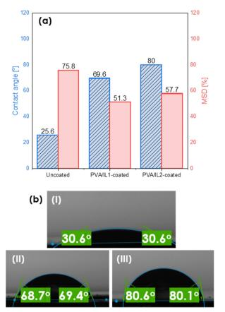
Fig. 7 Contact angle values (blue, dashed) and mass swelling degree (red, smooth) (a) and images of membrane surfaces taken during sessile drop tests for the uncoated (I) and PVA/IL1- (II) and PVA/IL2coated (III) membranes (b)
