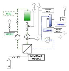
Fig. 1 Schematic representation of the pervaporation system, adopted from Annerl.<sup>30</sup>
