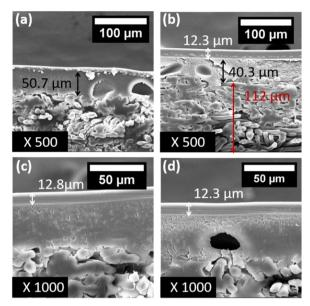
Fig. 3 SEM images at 500× magnification: uncoated membrane (a) and membrane coated with PVA/IL1 (b). SEM images at 1000× magnification: membrane coated with PVA/IL1 (c) and membrane coated with PVA/IL2 (d).
