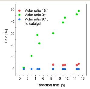
Fig. 11 Esterification-coupled pervaporation (T = 95 °C, sweep gas p= 3/2 bar (feed/permeate)) with the PVA/IL1-coated membrane and comparisons between different n-butanol/acetic acid molar ratios in
