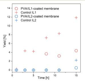
Fig. 10 Esterification comparison between PVA/IL1- and PVA/IL2coated membranes and control experiments (uncoated membrane, catalyst distributed in the reaction mixture) at T = 95 °C, sweep gas p= 3/2 bar (feed/permeate).
