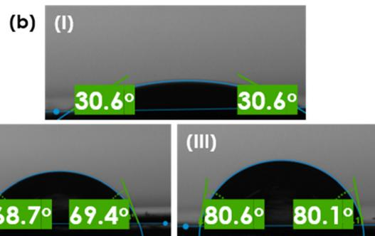
**Fig. 7** Contact angle values (blue, dashed) and mass swelling degree (red, smooth) (a) and images of membrane surfaces taken during sessile drop tests for the uncoated (I) and PVA/IL1- (II) and PVA/IL2-coated (III) membranes (b).
