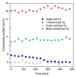
Fig. 8 Time evolution of the weight content [wt%] of each component of the feed mixture, for the membrane coated with PVA/ IL2 determined during esterification-coupled pervaporation at T = 95 $^{\circ}$ C, sweep gas p = 3/2 bar (feed/permeate).
