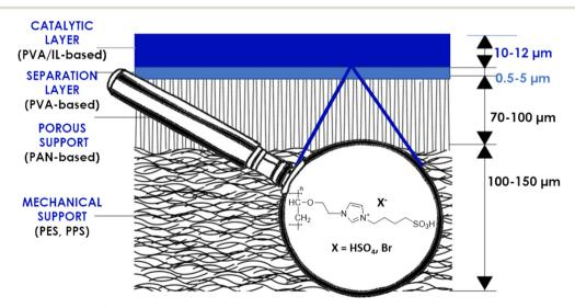
Fig. 2 Schematic representation of the coated membrane.
