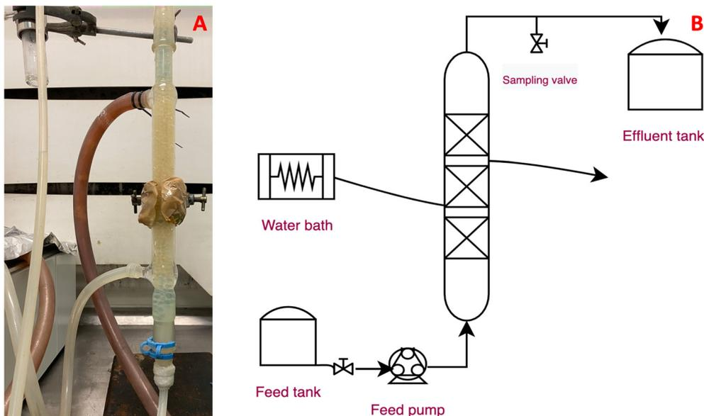
Fig. 2 The packed bed bioreactor: A photo of the experimental setup, B process flow diagram of the packed bed bioreactor.
