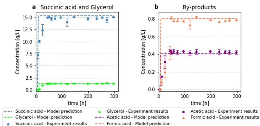
Fig. 7 Results for fermentation with initial substrate of  $15 \text{ g L}^{-1}$ , bioreactor length 20 cm and feed flow rate  $1.2 \text{ cm}^3 \text{ h}^{-1}$  ( $0.076 \text{ h}^{-1}$ ). (a): Succinic acid and glycerol concentration, (b): acetic and formic acid concentration.
