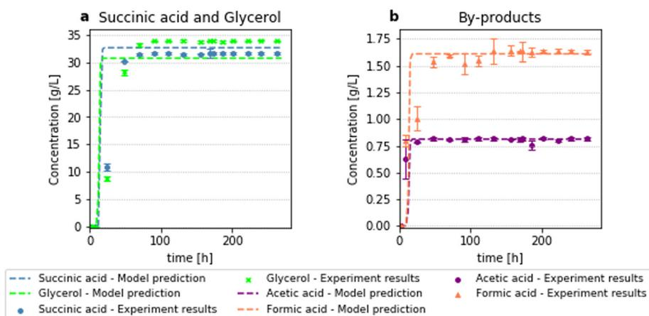
Fig. 8 Results for fermentation with initial substrate of  $60 \text{ g L}^{-1}$ , bioreactor length 40 cm and feed flow rate  $1.2 \text{ cm}^3 \text{ h}^{-1}$  ( $0.038 \text{ h}^{-1}$ ). (a): Succinic acid and glycerol concentration, (b): acetic and formic acid concentration.
