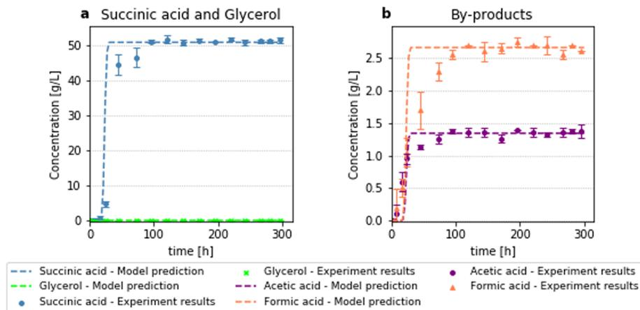
Fig. 14 Results for fermentation with optimal initial conditions: substrate of  $45 \text{ g L}^{-1}$ , and dilution rate  $0.042 \text{ h}^{-1}$ . (a): Succinic acid and glycerol concentration, (b): acetic and formic acid concentration.
