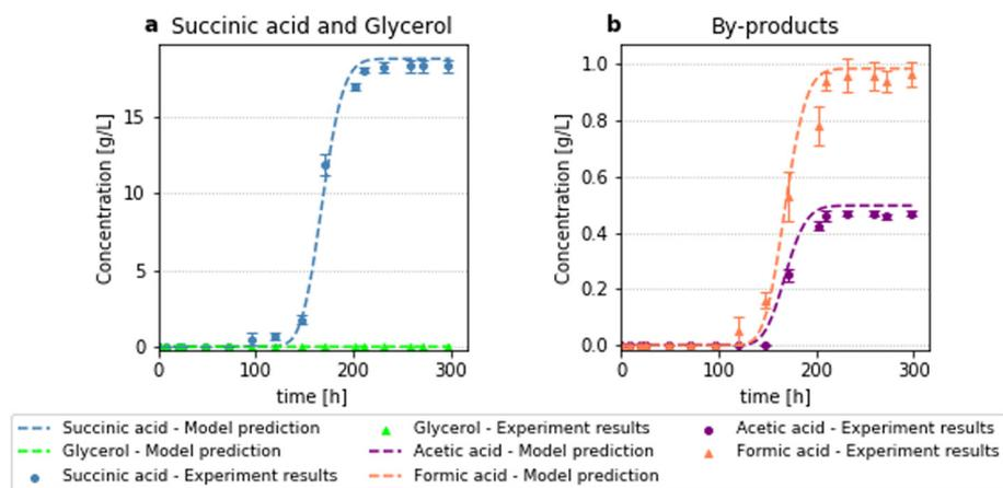
Fig. 6 Results for fermentation with initial substrate of  $15 \text{ g L}^{-1}$ , bioreactor length 40 cm and feed flow rate  $0.1 \text{ cm}^3 \text{ h}^{-1}$  ( $0.003 \text{ h}^{-1}$ ). (a): Succinic acid and glycerol concentration, (b): acetic and formic acid concentration.
