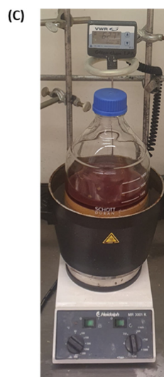
Fig. 1 Effects of solvents on the carbologation of 5-HMF (0.5 g) in 2.5 mL (a) dimethylcarbonate, (b) THF, (c) diethylether, (d) ethyl acetate, (e) dichloromethane, and (f) MIBK using TPT-Ome (1.1 mol%) as the catalyst at 40–60 °C. (A) Conversion of 5-HMF and yield of DHMF in the precipitate and solution. (B) Picture of the reaction solutions at 1 h. (C) Reaction at 400 g HMF scale in dimethyl carbonate. (D) DHMF purified from the reaction (C).
