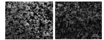
Fig. 10 SEM images of the (a) fresh catalyst and (b) spent catalyst.
