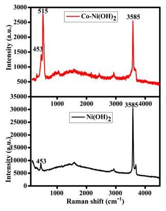
Fig. 3 Raman spectra of Co-Ni(OH)<sub>2</sub> and Ni(OH)<sub>2</sub>.
