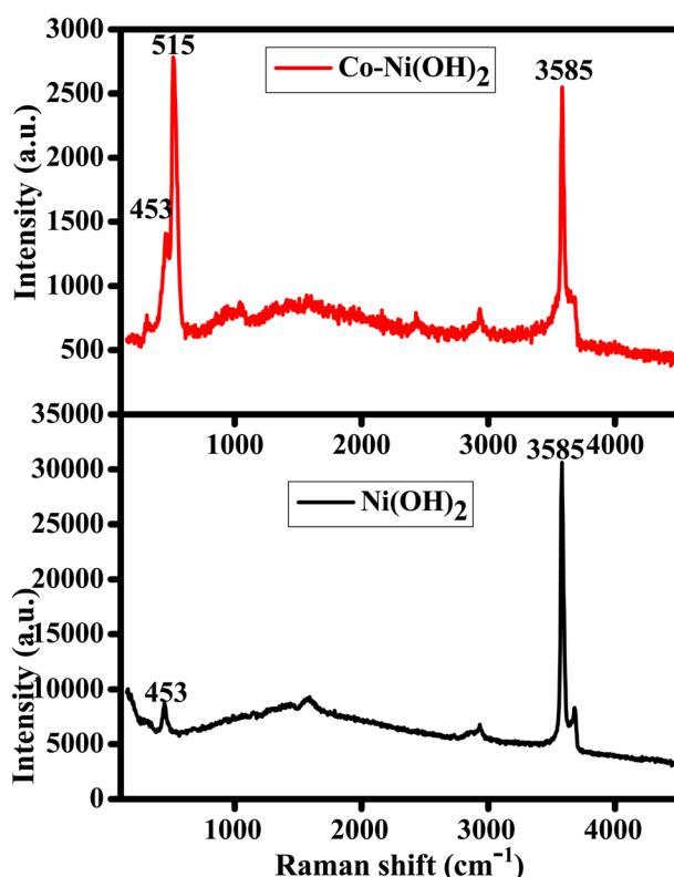
Fig. 3 Raman spectra of  $\text{Co-Ni(OH)}_2$  and  $\text{Ni(OH)}_2$ .
