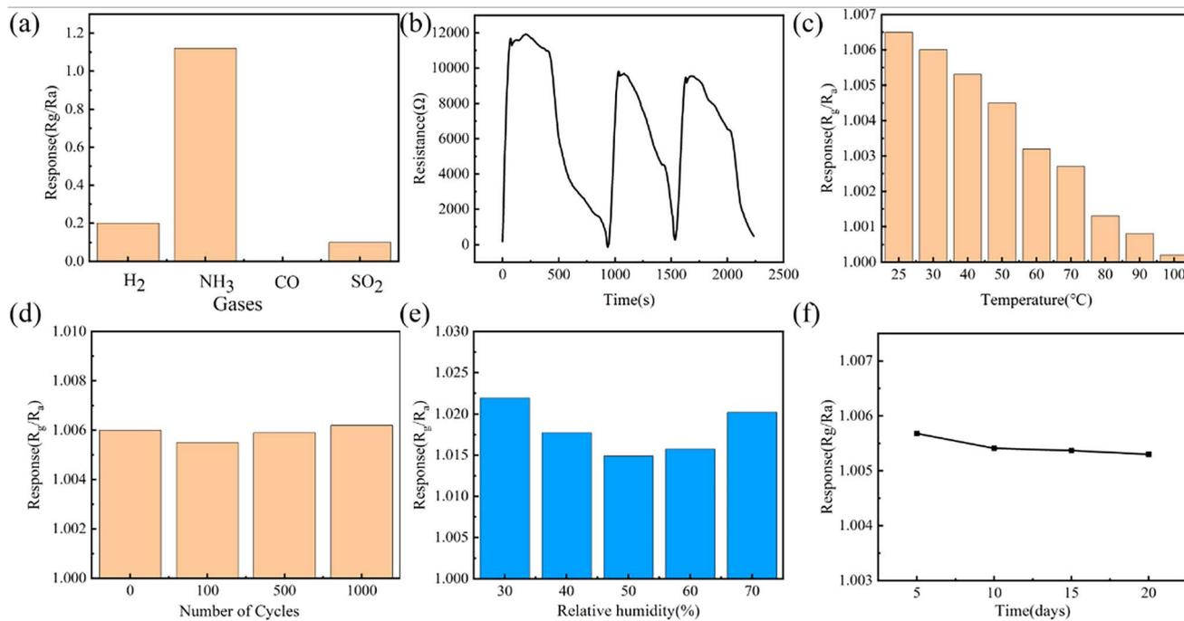
Fig. 7 (a) Response of fiber-shaped sensor towards different interference gases with a concentration of 40 ppm. (b) Cycling response toward 40 ppm NH<sub>3</sub> at room temperature. (c) Response value of the NH<sub>3</sub> sensor at different operating temperatures. (d) Response changes of NH<sub>3</sub> sensors after different bending cycles. (e) Response values of the NH<sub>3</sub> sensor at different relative humidities. (f) Temporal stability of the NH<sub>3</sub> sensors.
