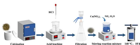
Fig. 1 Schematic illustration for the synthesis of CuSi-NTMs.
