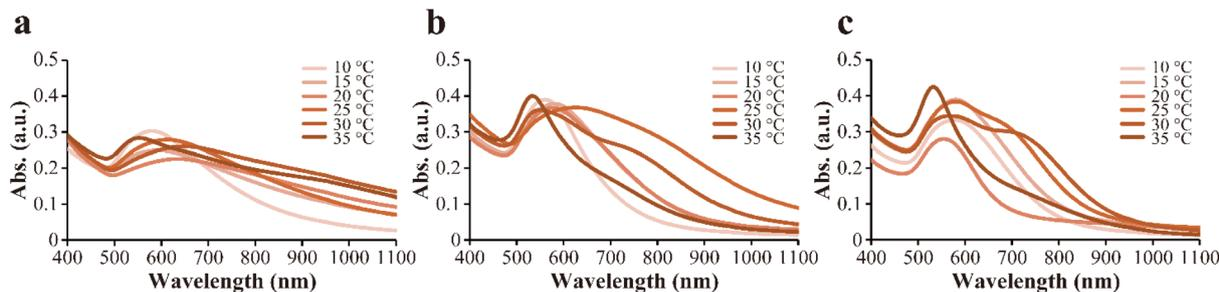
Fig. 5 (a–c) UV-vis spectra of samples after Au mineralization for 24 h using [Peptide] = 50  $\mu\text{M}$ , [HAuCl<sub>4</sub>] = 100  $\mu\text{M}$ , [AgNO<sub>3</sub>] = 50  $\mu\text{M}$  at 10–35 °C (a: W1; b: W2; c: W3).
