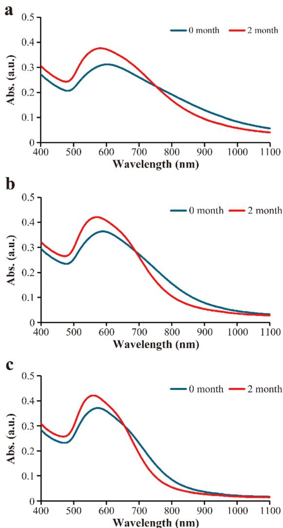
Fig. 3 UV-vis spectra of sample (Au nanostructures) immediately after mineralization and one month after mineralization using [Peptide] = 50  $\mu$ M, [HAuCl<sub>4</sub>] = 100  $\mu$ M, [AgNO<sub>3</sub>] = 50  $\mu$ M for 24 h at 20 °C (a: W1; b: W2; c: W3).
