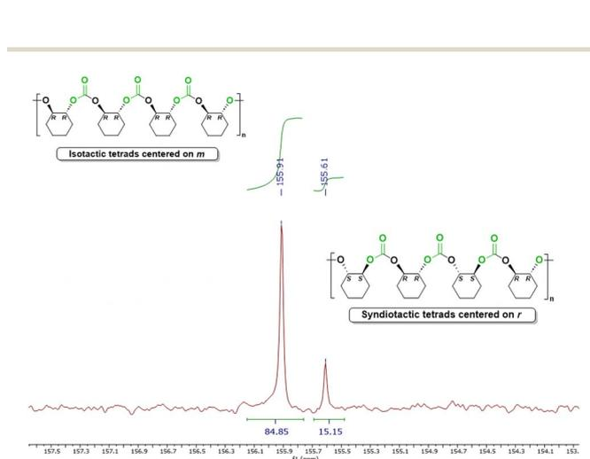
Fig. 2 Carbonyl region of the <sup>13</sup>C{<sup>1</sup>H} NMR spectrum in CDCl<sub>3</sub> of PCHC obtained using Cat5:DMAP.
