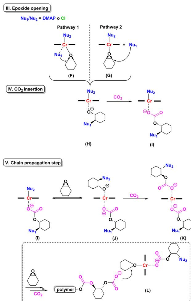
Scheme 4 Epoxide ring-opening through pathway 1 and pathway 2, followed by CO<sub>2</sub> insertion and chain propagation step, after consecutive CO<sub>2</sub> and CHO insertions.
