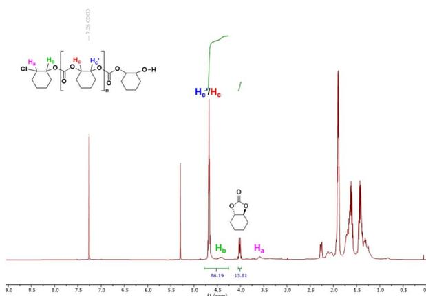
Fig. 1 <sup>1</sup>H NMR spectrum of PCHC obtained using Cat5:DMAP in CDCl<sub>3</sub>. Signals H<sub>a</sub> and H<sub>b</sub> are attributed to the terminal methine protons of the copolymer, while H<sub>c</sub>/H<sub>c'</sub> correspond to the methine protons within the copolymer backbone. Additionally, the signal at 4.0 ppm corresponds to 14% of the CHC-*trans*.
