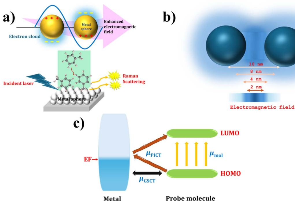
Fig. 1 Schematic illustration of (a) localized surface plasmon resonance and SERS effect *via* electromagnetic mechanism; (b) hot spots within small interparticle distance; (c) chemical enhancements in SERS.
