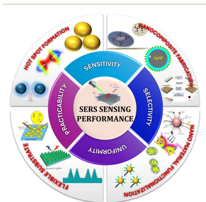
Fig. 2 Several main factors and strategies to improve SERS sensing performance. Illustration reproduced from ref. 38 with permission from the PCCP owner societies, copyright 2015; ref. 39 with permission from Springer Nature, copyright 2017; ref. 40 with permission from MPDI, copyright 2023; ref. 41 with permission from MPDI, copyright 2022; ref. 42 with permission from Elsevier, copyright 2019; ref. 43 with permission from MPDI, copyright 2021; ref. 44 with permission from The Royal Society of Chemistry copyright 2023; ref. 45 with permission from MPDI, copyright 2022; ref. 46 with permission Springer Nature, copyright 2017; ref. 47 with permission from The American Chemical Society, copyright 2015.
