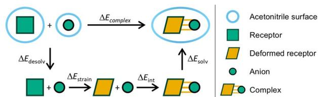
Fig. 6 Schematic representation of the coordination strength partitioning in solution. Since the anion is a single atom, no geometric deformation occurs for the anion.
