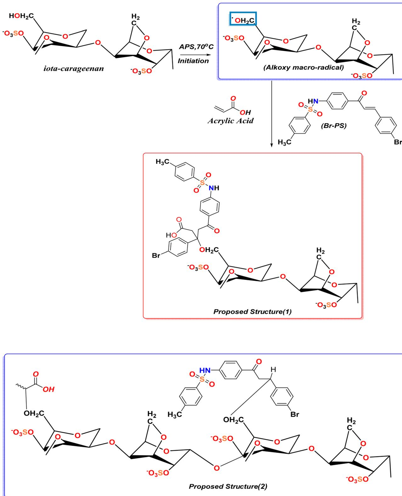
Scheme 1 Poly(Br-PS-co-AA)-g-carrageenan synthesis and its proposed structures.
