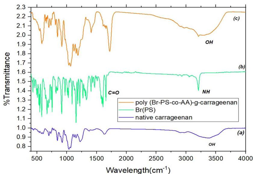
Fig. 1 FT-IR spectra for (a) native carrageenan, (b) Br-PS, and (c) poly(Br-PS-co-AA)-g-carrageenan.
