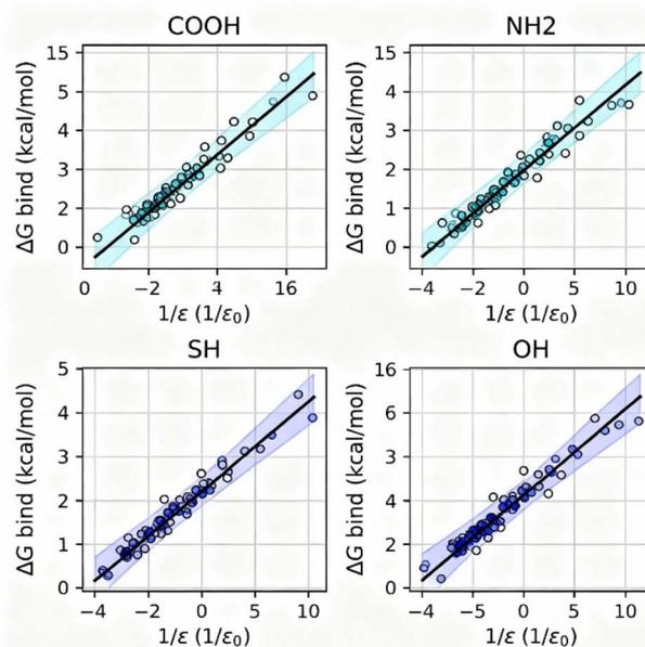
Fig. 2 Binding free energy ( $\Delta G_{\text{bind}}$ ) *versus* inverse dielectric constant ( $1/\epsilon$ ) for each functional group with experimental data, regression lines, and 95% confidence intervals.
