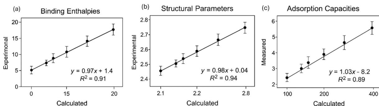
Fig. 5 Validation of computational results against experiments: (a) calculated vs. experimental binding enthalpies from ITC and TPD; (b) Cd–O coordination distances from EXAFS; (c) predicted vs. measured Cd $^{2+}$  adsorption capacities of functionalized MOFs in aqueous media.
