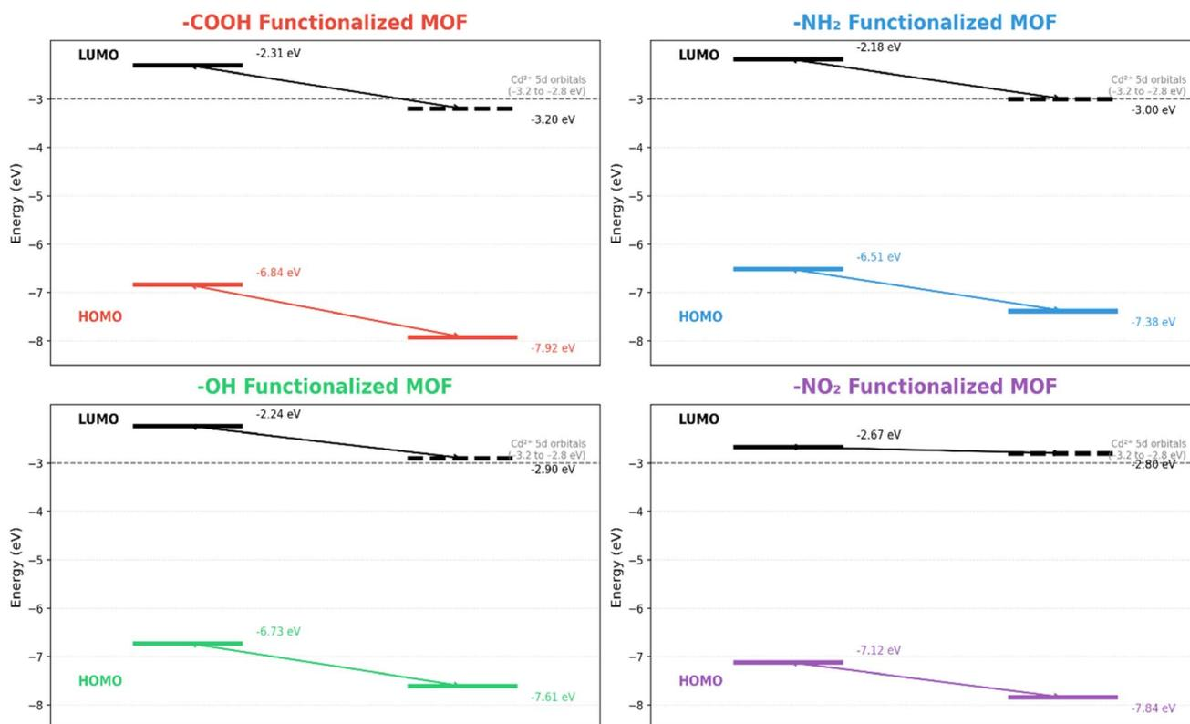
Fig. 3 HOMO–LUMO energy diagrams of functionalized MOFs before and After Cd<sup>2+</sup> coordination.
