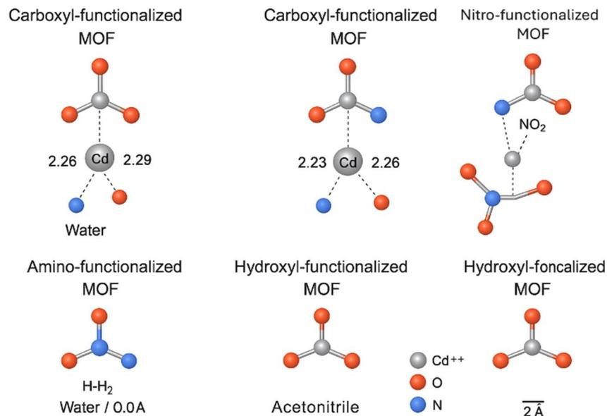
Fig. 1 Optimized structures of  $\text{Cd}^{2+}$ -MOF complexes for each functional group in water and acetonitrile, with labeled bond distances.
