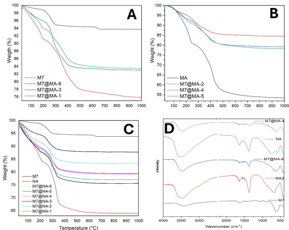
Fig. 6 TGA graphics for core@shell solids containing MA LDH (A and B), core@shell solids containing NA LDH (C) and FTIR spectra for core@shell solids, besides the MA and NA LDHs and M7 (D).
