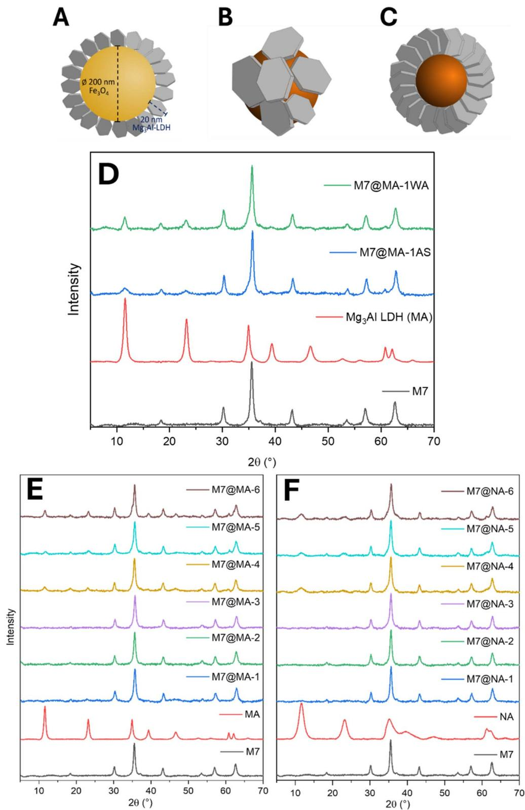
**Fig. 3** Idealized core@shell solid representation with 200 nm core and 20 nm shell sizes (A) and representation of LDH/magnetite assemblies for  $\text{M7@MA-6}$  (B) and  $\text{M7@NA-4}$  (C), (D) diffractograms for core@shell prepared by the proposed route using the solid M7 as core and  $\text{Mg}_3\text{Al-LDH}$  (MA) as shell and the diffractograms for core@shell solids prepared varying the LDH/magnetite molar ratio from 0.1 to 0.6, for the MA-LDH (E) and NA-LDH (F) series.
