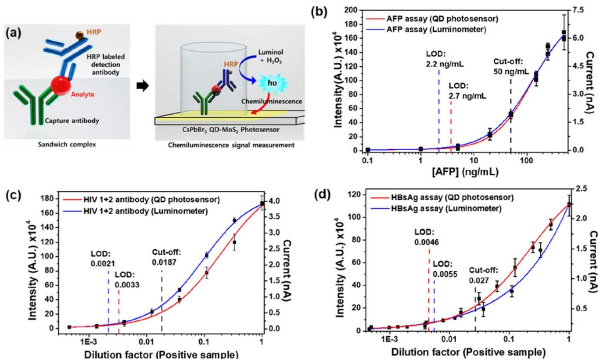
Fig. 4 (a) Schematic of CsPbBr<sub>3</sub> QD-MoS<sub>2</sub> photosensor for chemiluminescence detection. (b) AFP detection intensity with photosensor and luminometer. (c) Anti-HIV antibody detection intensity vs. dilution. (d) HBsAg detection intensity vs. dilution. Adapted with permission from ref. 103, Copyright 2021 American Chemical Society.
