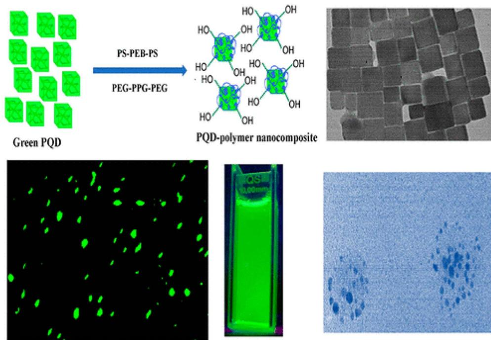
Fig. 2 Water-soluble CsPbBr<sub>3</sub> PQD-polymer nanocomposites formed by dual encapsulation with PS-PEB-PS and PEG-PPG-PEG, showing preserved cubic morphology (TEM), bright green emission under UV, and selective anti-CD63-mediated labeling of triple-negative breast tumor-derived exosomes. Adapted with permission from ref. 89, Copyright 2019 American Chemical Society.
