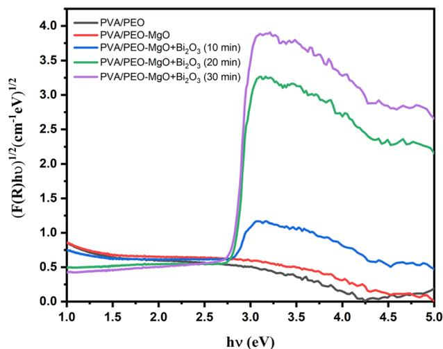
Fig. 5 Relationship between  $(F(R)hv)^{1/2}$  and the photon energy  $h\nu$  for PVA/PEO, PVA/PEO–MgO, and PVA/PEO–MgO– $\text{Bi}_2\text{O}_3$  nanocomposites.
