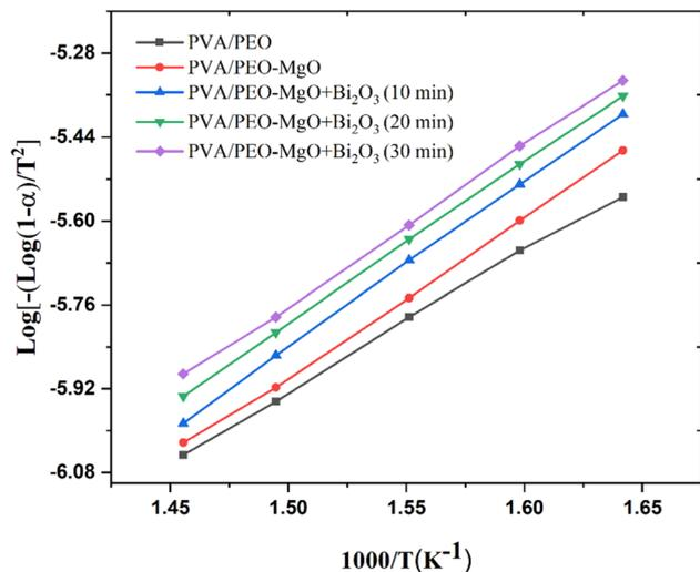
Fig. 8 Relation between  $-\log\left[\frac{-\log(1-\alpha)}{T^2}\right]$  against reciprocal temperature  $\left(\frac{1000}{T}\right)$  for PVA/PEO, PVA/PEO-MgO, and PVA/PEO-MgO-Bi<sub>2</sub>O<sub>3</sub> nanocomposites.
