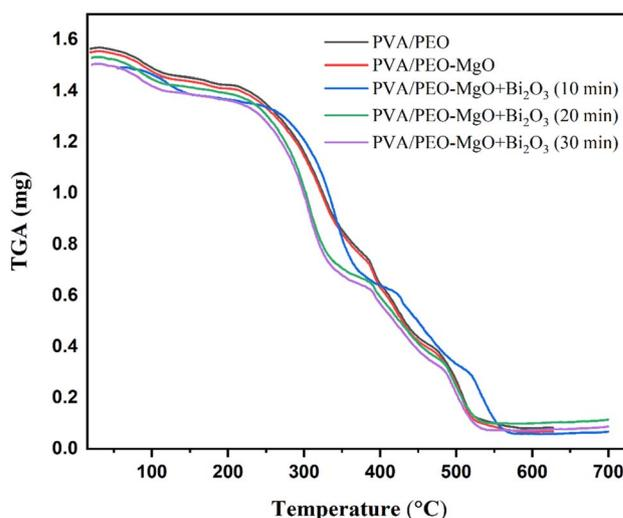
Fig. 7 TGA thermograms for PVA/PEO, PVA/PEO–MgO, and PVA/PEO–MgO–Bi<sub>2</sub>O<sub>3</sub> nanocomposites.
