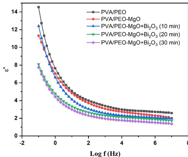
Fig. 9 Variation of the dielectric constant ( $\epsilon'$ ) as a function of  $\log f$  for PVA/PEO, PVA/PEO-MgO, and PVA/PEO-MgO-Bi<sub>2</sub>O<sub>3</sub> nanocomposites.
