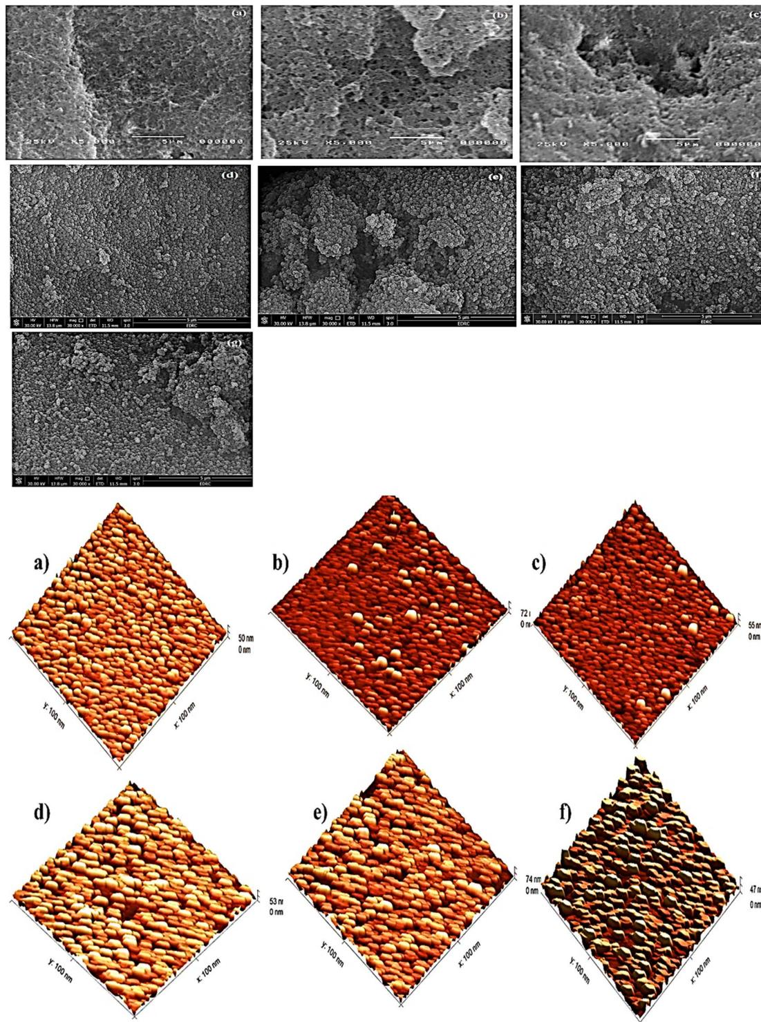
**Fig. 4** (A): SEM images of (a) MIP (B) unwashed, (b) MIP (B) washed, (c) NIP (B), (d) bare silica, (e) MIP (S) washed, (f) MIP (S) unwashed, and (g) NIP (S). (B): AFM 3D images for (a) unwashed MIP (B), (b) washed MIP (B), (c) NIP (B), (d) unwashed MIP (S), (e) washed MIP (S), and (f) NIP (S).
