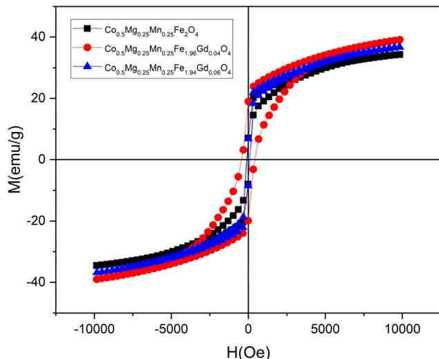
Fig. 7 Magnetization ( $M$ ) versus applied magnetic field ( $H$ ) curves at room temperature for  $\text{Co}_{0.5}\text{Mn}_{0.25}\text{Mg}_{0.25}\text{Fe}_{2-x}\text{Gd}_x\text{O}_4$  nanoparticles with different  $\text{Gd}^{3+}$  concentrations ( $x = 0.00, 0.04, 0.06$ ).
