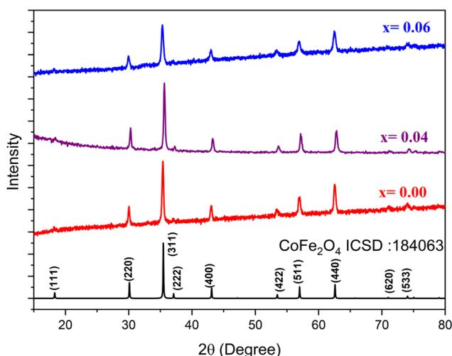
Fig. 1 X-ray diffraction patterns of  $\text{Co}_{0.5}\text{Mn}_{0.25}\text{Mg}_{0.25}\text{Fe}_{2-x}\text{Gd}_x\text{O}_4$  ( $x = 0.00, 0.04, 0.06$ ) nanoparticles.
