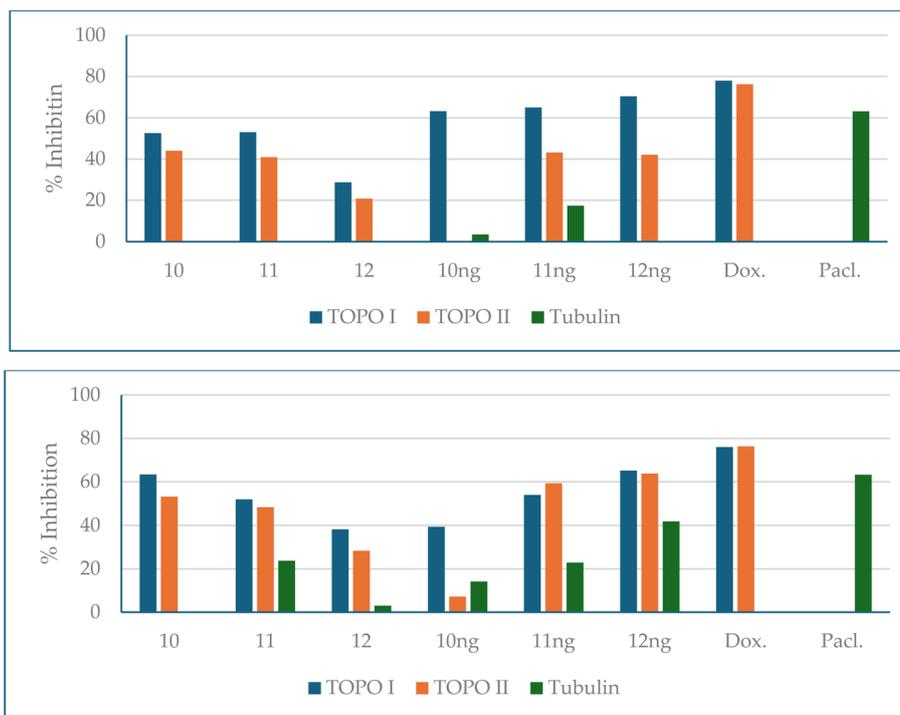
Fig. 8 Mean % inhibition activity of compounds 10–12, their nanogel formulations (10ng–12ng), and reference agents on TOPO I, II, and tubulin in Caco2 (upper panel) and MDA-MB-231 (lower panel).
