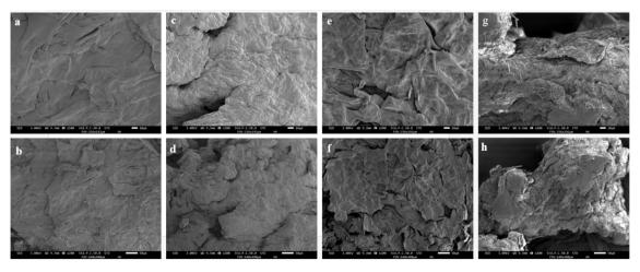
Fig. 4 SEM images of CGT before extraction and after extraction (the extraction conditions were: L/S = 1:66, 20% V/V, water 61 °C, 39 min). a and b Are unprocessed medicinal powders. c and d Are extracted after water extraction. e and f Are extracted after methanol extraction. g and h Are extracted from Choline chloride-levulinic acid.
