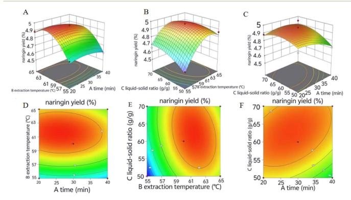
Fig. 3 The three-dimensional (3D) plots and two-dimensional (2D) as a function of extraction time, solid-liquid ratio, and water content in extraction temperature.
