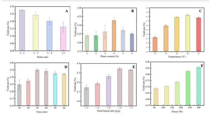
Fig. 2 Contents of extraction of naringin with ChCl-Le (1:2) from CGE. (A) Effect of the molar ratio of ChCl-Le, (B) water content in NADES/ water solution, (C) extraction temperature, (D) extraction time, (E) solid/liquid ratios (F) power on extracted amounts of naringin from CGE using UAE. Error bars indicate the relative standard deviation (n = 3).
