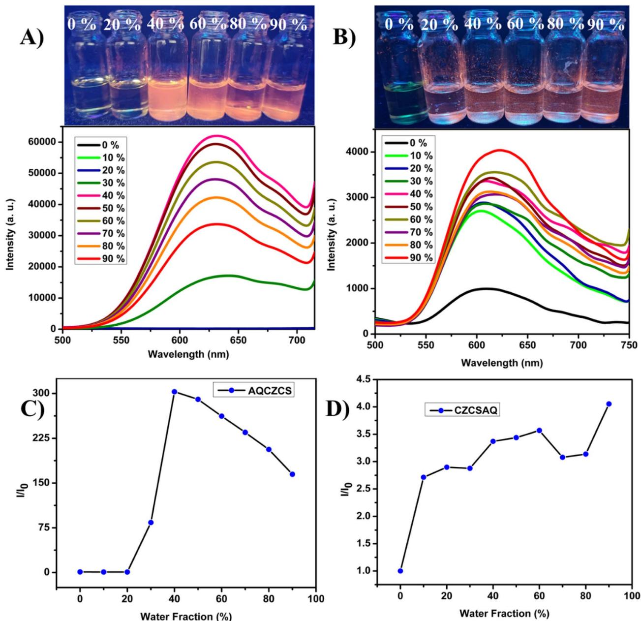
Fig. 2 Fluorescence spectra of (A) AQCZCS and (B) CZCSAQ in DMSO-water mixtures with different water fractions. Digital photos taken for the various water fractions under UV 365 nm lamp are displayed at the top of the spectra.  $I/I_0$  plots of (C) AQCZCS and (D) CZCSAQ with different fractions of water (Con. 10  $\mu$ M,  $\lambda_{\text{ex}} = 380$  nm for AQCZCS and  $\lambda_{\text{ex}} = 400$  nm for CZCSAQ). (Instrumental parameters: excitation slit width and emission slit width = 20 nm).
