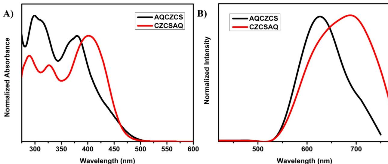
Fig. 1 (A) Normalized absorption and (B) normalized emission spectra of isomers **AQCZCS** and **CZCSAQ** in THF (Con. 10  $\mu$ M,  $\lambda_{\text{ex}}$  = 380 nm for **AQCZCS** and  $\lambda_{\text{ex}}$  = 400 nm for **CZCSAQ**).
