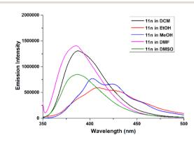
Fig. 1 Emission spectra in various organic solvents for compound 11n.
