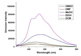
Fig. 4 Emission spectra in various organic solvents for compound 17.
