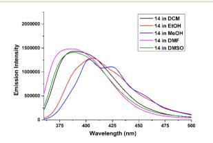
Fig. 2 Emission spectra in various organic solvents for compound 14.
