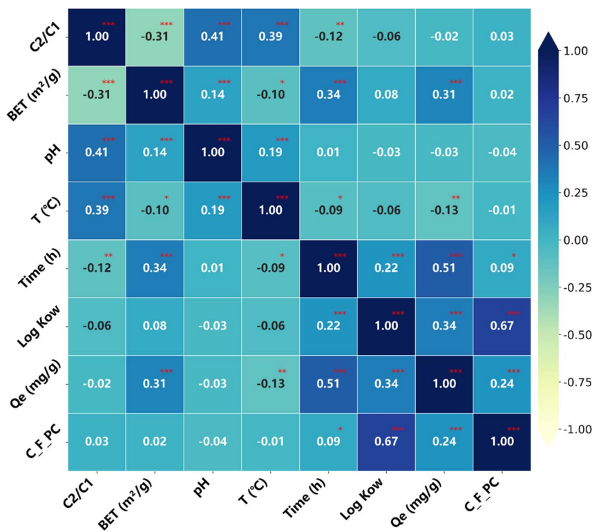
Fig. 3 Pearson correlation matrix of the selected features and the adsorption capacity. The color scale is fixed between -1 and 1 , where the color intensity represents the strength and sign of the linear correlation ( -1 : strong negative, +1 : strong positive, 0 : weak or no correlation). The numbers in each cell denote the Pearson correlation coefficients ( r ), while the star symbols indicate the statistical significance levels based on the corresponding p -values ( *p < 0.05 , **p < 0.01 , ***p < 0.001 ).
