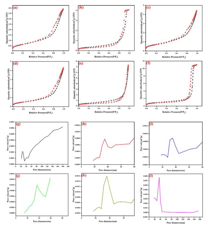
Fig. 5  $N_2$  adsorption-desorption isotherms (a) NFO, (b) SnO<sub>2</sub>, (c) CeO<sub>2</sub>, (d) NFO/SnO<sub>2</sub>, (e) NFO/CeO<sub>2</sub>, (f) NFO/SnO<sub>2</sub>/CeO<sub>2</sub>, with its pore size distribution plot of (g) NFO, (h) SnO<sub>2</sub>, (i) CeO<sub>2</sub>, (j) NFO/SnO<sub>2</sub>, (k) NFO/CeO<sub>2</sub>, (l) NFO/SnO<sub>2</sub>/CeO<sub>2</sub> for the synthesised materials.
