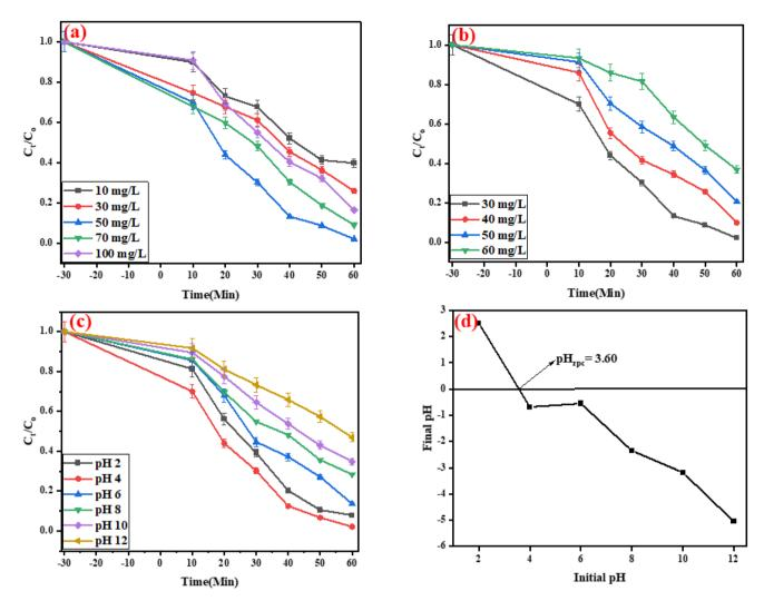
Fig. 11 (a) Effect of dosage plot, (b) effect of TCN concentration, (c) effect of pH and (d) point of zero charge ( $pH_{zpc}$ ) using the ternary nanocomposite NFO/SnO<sub>2</sub>/CeO<sub>2</sub> catalyst.
