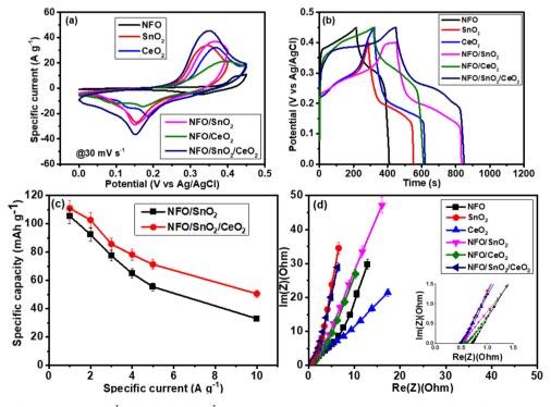
Fig. 7 Comparison of (a) CV at 30 mV s<sup>-1</sup>, (b) GCD at 1 A g<sup>-1</sup>, (c) specific capacity *versus* specific current of NFO/SnO<sub>2</sub> and NFO/SnO<sub>2</sub>/CeO<sub>2</sub>, (d) Nyquist plot (with an inset at high frequency).
