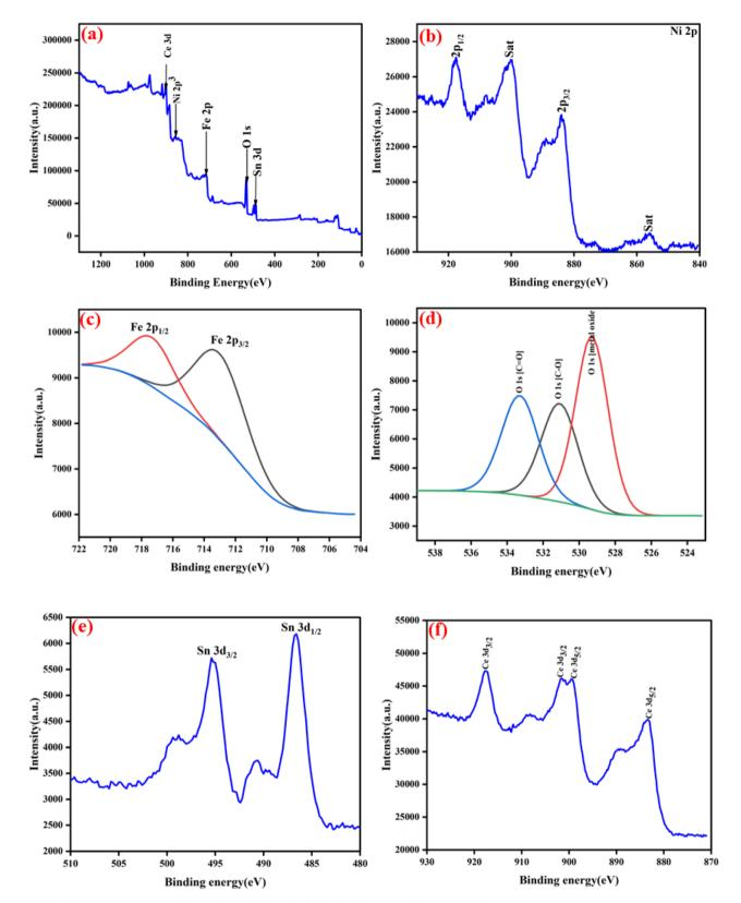
Fig. 4 (a) XPS survey scan of NFO/SnO<sub>2</sub>/CeO<sub>2</sub>, (b) Ni 2p, (c) Fe 2p, (d) O 1s, (e) Sn 3d, and (f) Ce 3d.
