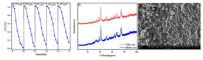
Fig. 12 (a) Cycling test for the photocatalytic degradation of TCN (b) XRD patterns of the fresh and used and (c) SEM image of the NFO/SnO $_2$ /CeO $_2$  nanocomposite.
