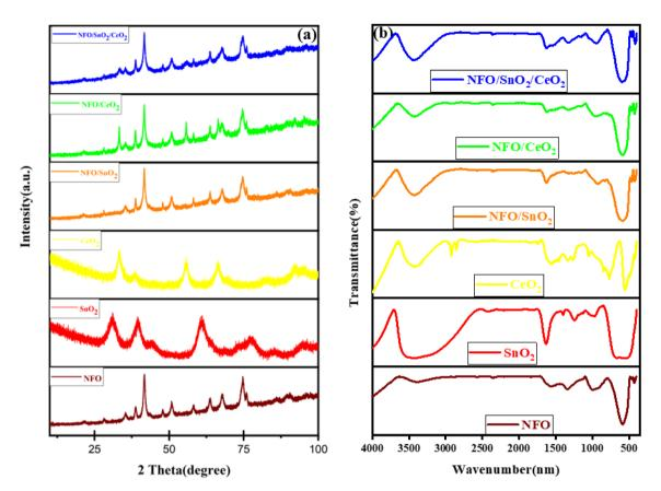
Fig. 1 (a) XRD and (b) FTIR patterns of pristine NFO, SnO<sub>2</sub>, CeO<sub>2</sub> and NFO-based photocatalysts.
