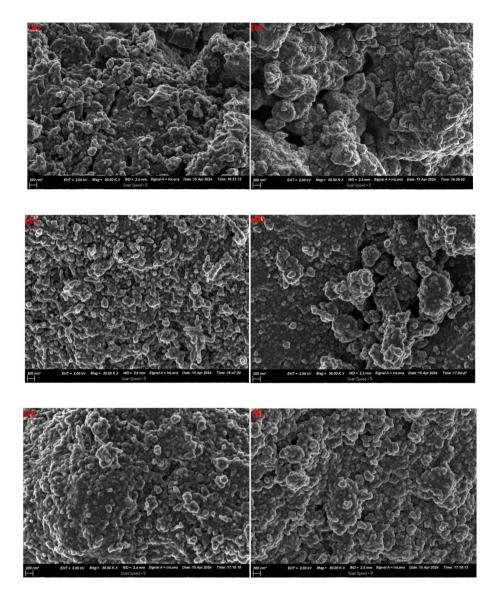
Fig. 2 SEM images of the as-prepared samples: (a) NiFe<sub>2</sub>O<sub>4</sub>, (b) SnO<sub>2</sub>, (c) CeO<sub>2</sub>, (d) NiFe<sub>2</sub>O<sub>4</sub>/SnO<sub>2</sub>, (e) NiFe<sub>2</sub>O<sub>4</sub>/CeO<sub>2</sub> and (f) nanocomposite NiFe<sub>2</sub>O<sub>4</sub>/SnO<sub>2</sub>/CeO<sub>2</sub>.
