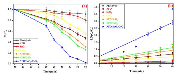
Fig. 9 (a) Photocatalytic degradation of TCN and (b) pseudo-first-order kinetics of TCN degradation over the synthesised composite materials.
