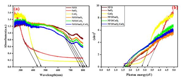
Fig. 6 (a) UV-vis diffuse reflectance spectroscopy spectra and (b) Tauc plots of the synthesised materials
