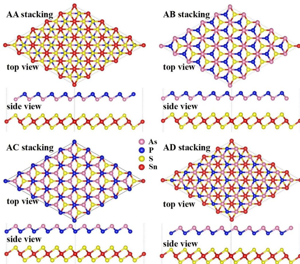
Fig. 1 Relaxed structures ( $5 \times 5$  supercell) of the four typical stacking patterns of the AsP/SnS<sub>2</sub> heterostructure.
