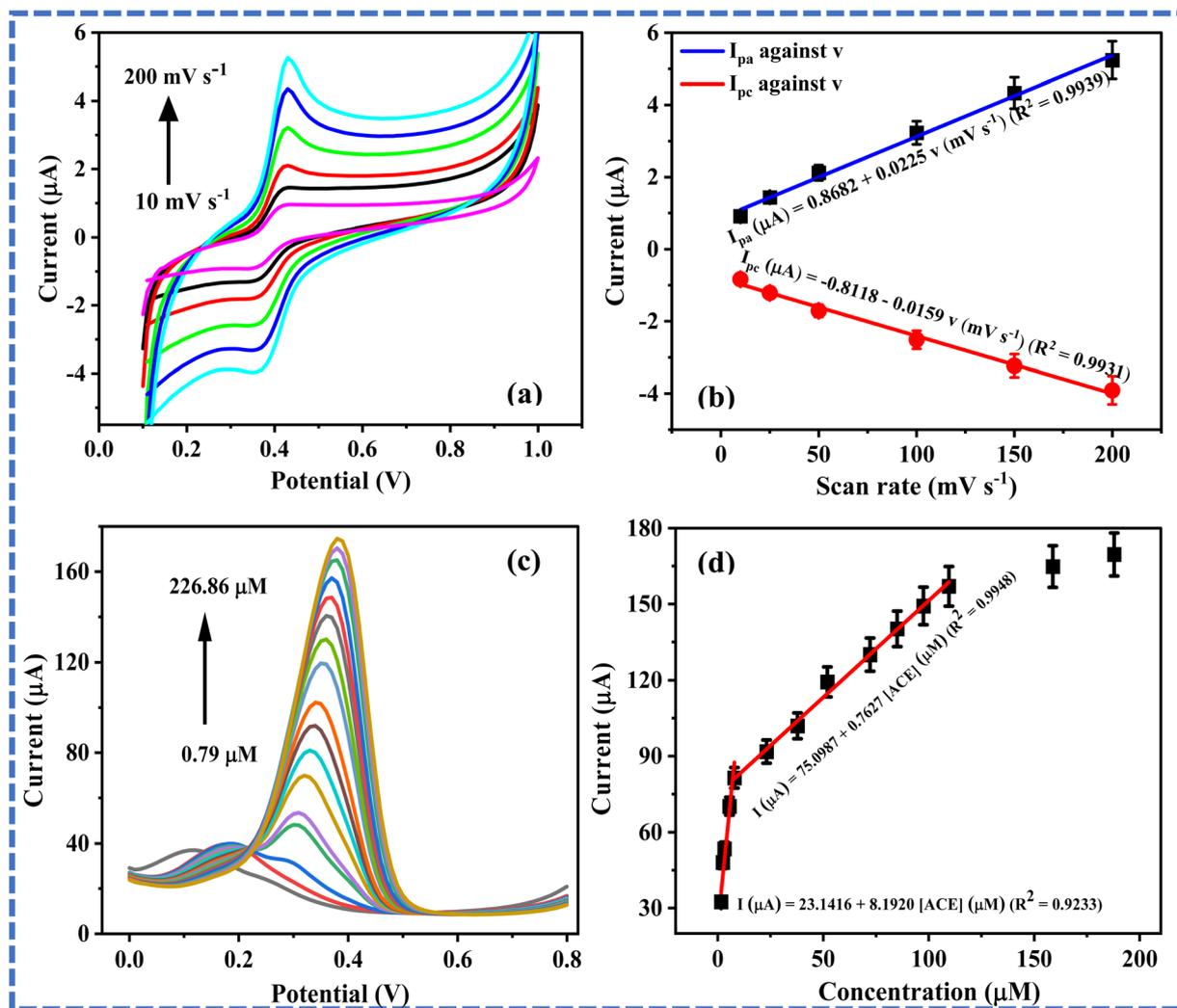
Fig. 4 (a) Cyclic voltammograms of  $75 \mu\text{M}$  ACE over a scan rate range of  $25\text{--}450 \text{ mV s}^{-1}$  (pH 5.23), (b) plot of peak current against scan rate, (c) differential pulse voltammograms of varying ACE concentrations ( $0.79\text{--}226.86 \mu\text{M}$ ) at EPM/GCE, and (d) plot of ACE peak currents against concentration.
