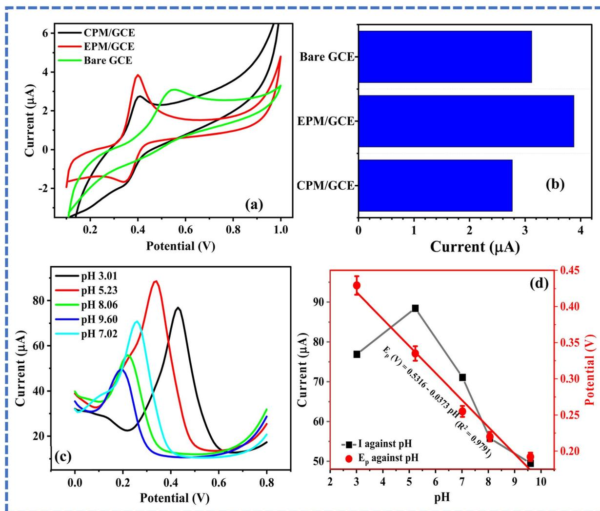
Fig. 3 (a) Cyclic voltammograms of 0.16 mM ACE at bare GCE, CPM/GCE and EPM/GCE. (b) Chart showing the peak currents recorded from (a). (c) Differential pulse voltammogram of 15  $\mu$ M ACE at EPM/GCE in phosphate buffer of varying pH (3.01–9.6) and (d) plots of ACE peak current and corresponding peak potentials against buffer pH.
