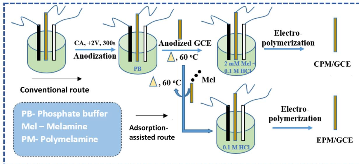
Scheme 1 Fabrication of PM-modified electrode via the conventional and adsorption-assisted electropolymerization methods.
