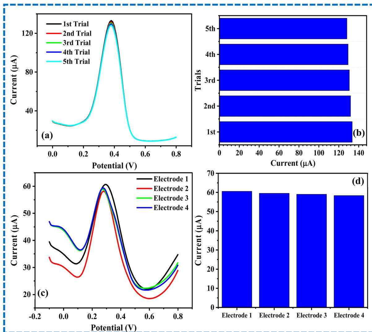
Fig. 8 (a) Differential pulse voltammograms of 85  $\mu\text{M}$  ACE over EPM/GCE recorded five times, and (b) chart showing the peak currents recorded in (a). (c) Differential pulse voltammograms of 10  $\mu\text{M}$  ACE over four different EPM/GCE, and (d) chart showing the peak currents recorded in (c).
