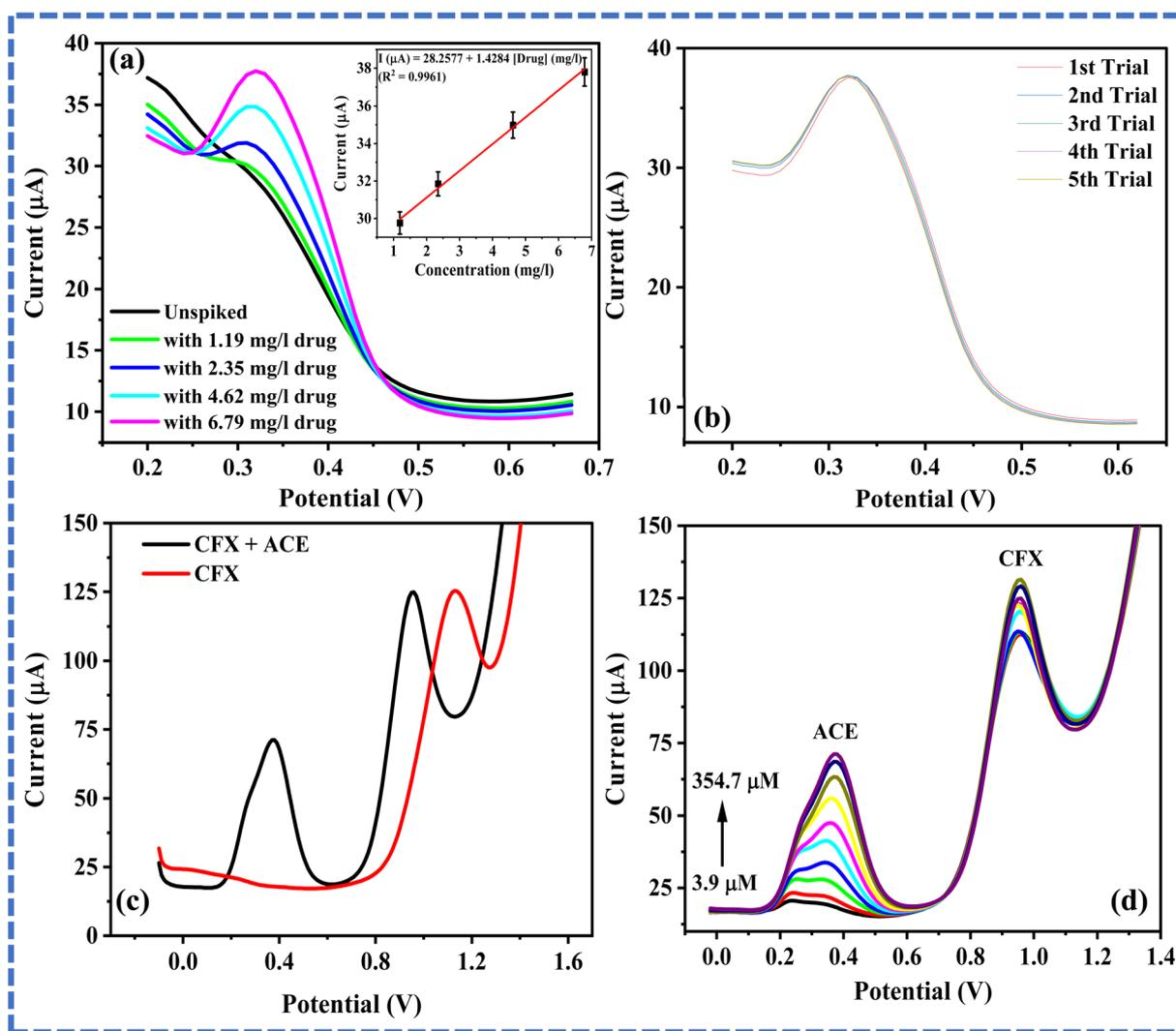
Fig. 5 Differential pulse voltammogram of (a) unspiked tap water and tap water spiked with 1.19–6.79  $\text{mg L}^{-1}$  drug (inset: plot of peak current against concentration of drug), (b) 6.8  $\text{mg L}^{-1}$  drug (recorded five times), (c) 1 mM CFX and a mixture of 350  $\mu\text{M}$  ACE and 1 mM CFX at EPM/GCE (pH 5.23), and (d) varying ACE concentrations (3.9–354.7  $\mu\text{M}$ ) in the presence of 1 mM CFX.
