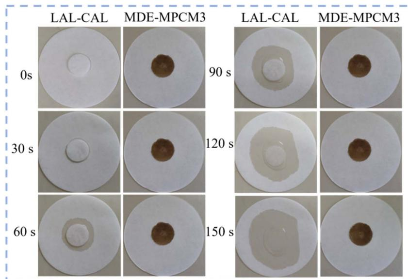
Fig. 9 The leakage photographs of LAL-CAL and MDE-MPCM3.
