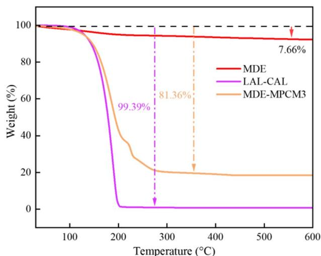
Fig. 8 The TGA curves of MDE-MPCM3.
