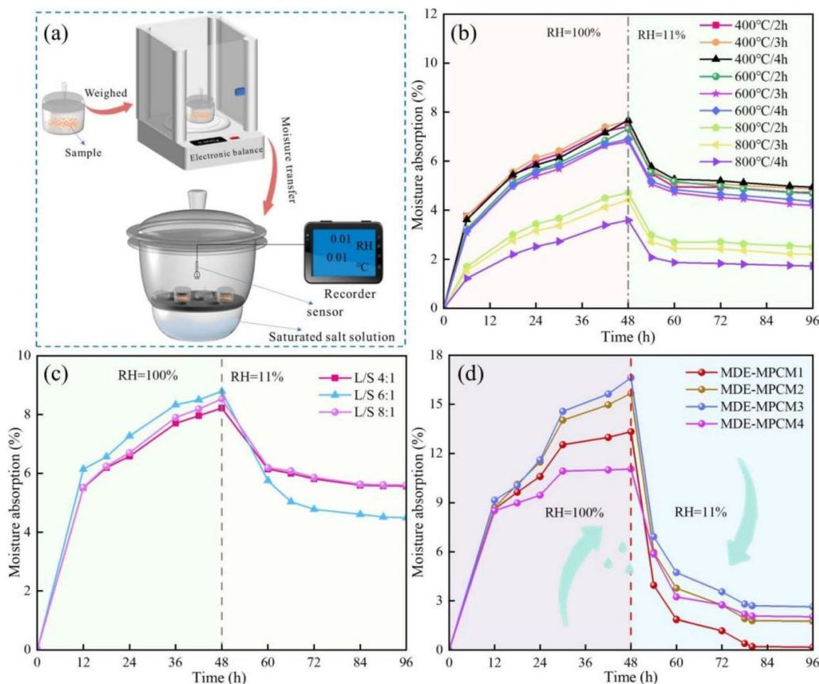
Fig. 5 Scheme of the experimental setup of (a) and the influence of different calcination conditions (b) and L/S ratio (c), (d) humidity control performance of the samples.
