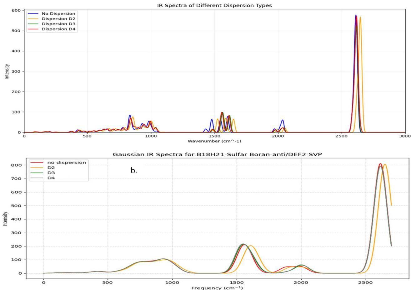
Fig. 3 Calculated IR spectrum for borane: (a) 1HS-B<sub>18</sub>H<sub>21</sub>-syn forgotten and, (b) 4HS-B<sub>18</sub>H<sub>21</sub>-anti with dispersion types.
