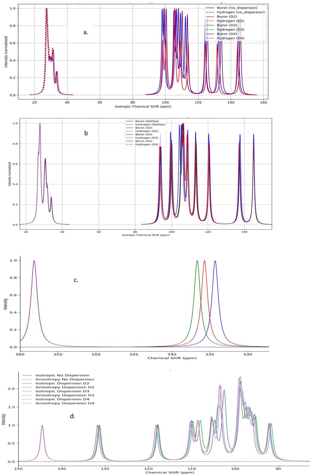
Fig. 9 NMR – chemical shift spectra for (a)  $B_{18}H_{22}$ -syn and (b)  $B_{18}H_{22}$ -anti, (c) 1HS- $B_{18}H_{21}$ -syn and (d) 4HS- $B_{18}H_{21}$ -anti.
