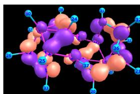
figure 12.h. LUMO D4/ for  $B_{18}H_{22}$  - *anti*
