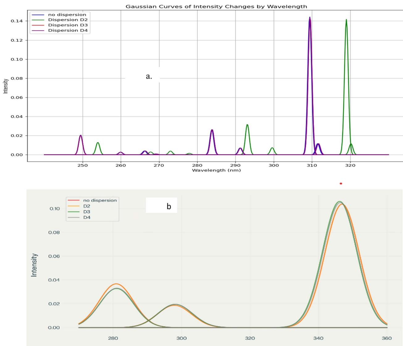
**Fig. 4** (a) UV-Vis spectra for B<sub>18</sub>H<sub>22</sub> *syn* 'forgotten' with dispersion types. (b) UV-Vis spectra for B<sub>18</sub>H<sub>22</sub> *anti* with dispersion types.
