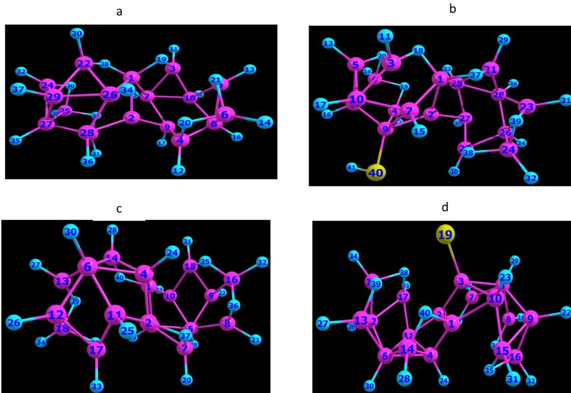
Fig. 1 Optimized BP86/def2-svp geometries of: (a) B<sub>18</sub>H<sub>22</sub>-*syn* isomer, (c) B<sub>18</sub>H<sub>22</sub>-*anti* isomer, (b) [1-HS-*syn*-B<sub>18</sub>H<sub>21</sub>] and (d) [4-HS-*anti*-B<sub>18</sub>H<sub>21</sub>] isomers. Yellow color denotes a sulfur substituent.
