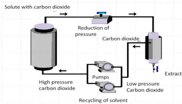
Fig. 6 Annotated diagram of super-critical fluid extraction process.<sup>54</sup>
