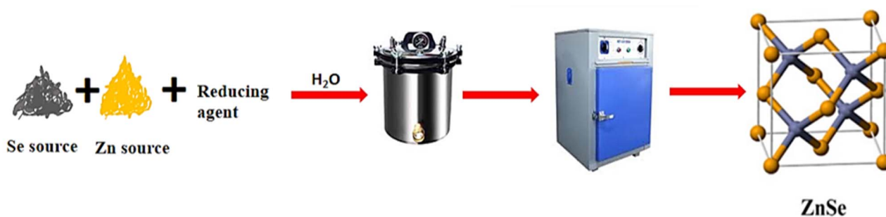
Fig. 4 Schematic representation of a hydrothermal method for the synthesis of zinc selenides (reproduced from ref. 60).
