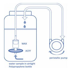
Fig. 5 Schematic of the in situ SPE set-up. 120
