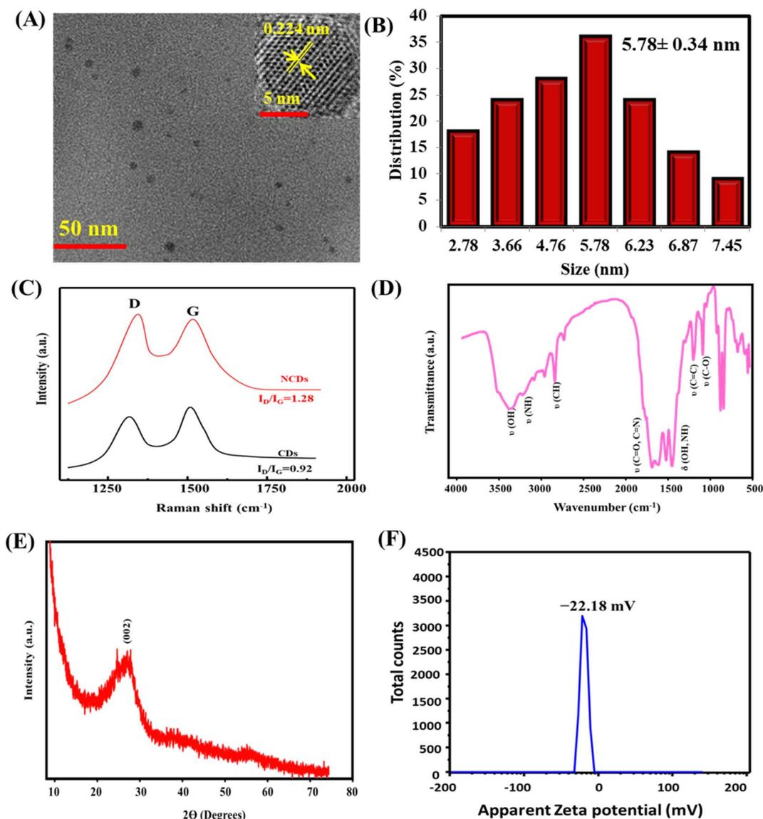
Fig. 1 SEM (A), size distribution (B), Raman spectra (C), FTIR (D), XRD (E), and zeta potential (F) of biowaste-derived NCDs. Raman spectrum of CDs is provided in (C) for comparison. The zeta potential was carried out in ultrapure water.
