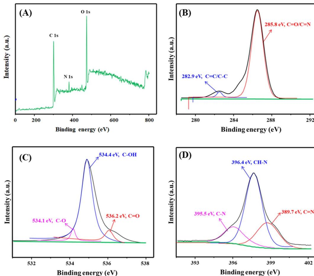
Fig. 2 (A) Full XPS survey of biowaste-derived NCDs; (B–D) deconvoluted spectra of C 1s, O 1s, and N 1s, respectively.
