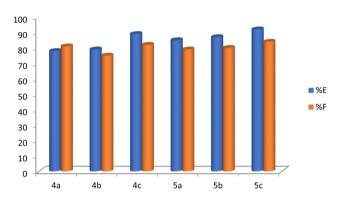
Fig. 6 Percentages of polyester fabric dye fixation and exhaustion.
