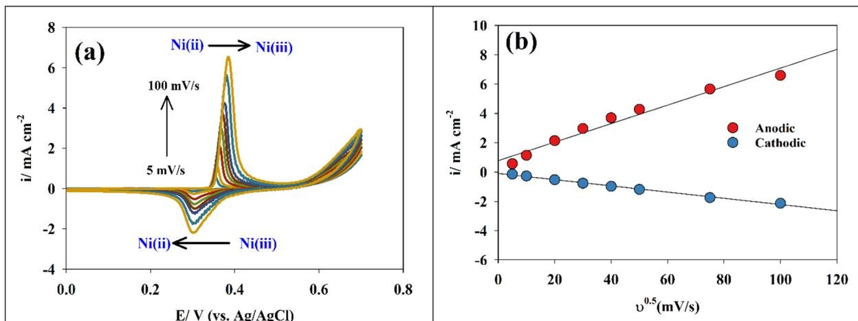
Fig. 4 (a) CVs of NCO-ZIF-8B at various scan rate ranges (5–100 mV s<sup>-1</sup>), (b) linear relation between scan rate and current density.
