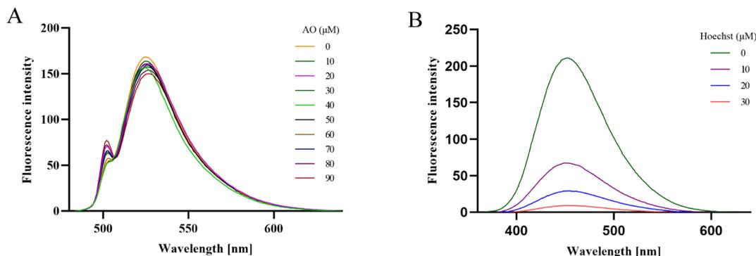
Fig. 2 Competitive displacement assays demonstrating the binding specificity of IMDP-DNA. (A) Fluorescence spectra of the Ct-DNA (50  $\mu\text{M}$ ) and AO (5  $\mu\text{M}$ ) complexes in the presence of varying concentrations of IMDP (0–90  $\mu\text{M}$ ). (B) Fluorescence spectra of Ct-DNA (50  $\mu\text{M}$ ) and the Hoechst 33258 (5  $\mu\text{M}$ ) complex in the presence of varying concentrations of IMDP (0–30  $\mu\text{M}$ ).
