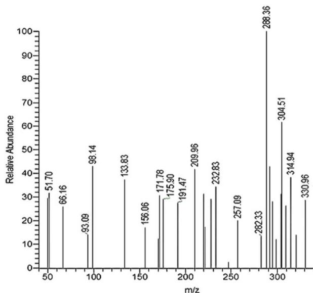
Fig. 3 ESI-MS spectrum of the pyrazolone–thiophene Schiff base (PyTh). The spectrum shows the molecular ion  $[M + H]^+$  at  $m/z$  329.05 (calc. for  $C_{15}H_{13}N_4OS_2$ ) appearing with low intensity. The base peak at  $m/z$  288.36 corresponds to a major fragment, indicating significant in-source fragmentation.
