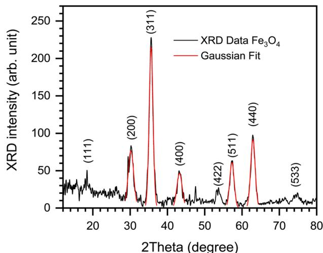
Fig. 6 XRD pattern of Fe<sub>3</sub>O<sub>4</sub> nanoparticles with Gaussian fit overlay, highlighting major indexed reflections at (220), (311), (400), (511), and (440).
