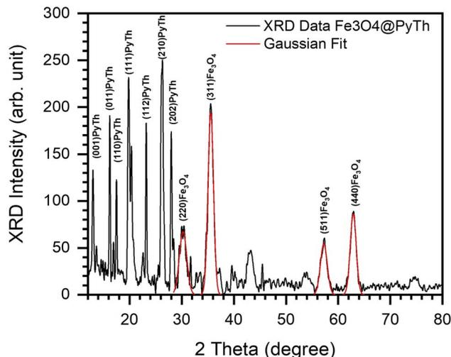
Fig. 7 XRD pattern of the  $\text{Fe}_3\text{O}_4@PyTh$  nanocomposite, showing PyTh-specific reflections alongside core  $\text{Fe}_3\text{O}_4$  peaks.
