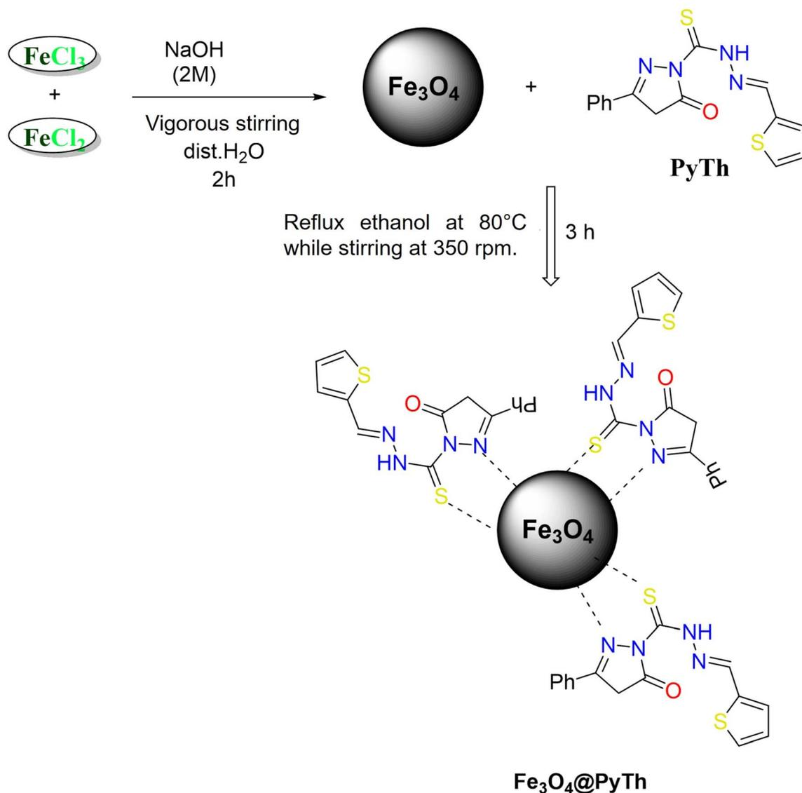
Scheme 2 Anchoring of the pyrazolone Schiff base (PyTh) on the surface of Fe<sub>3</sub>O<sub>4</sub> magnetic nanoparticles.
