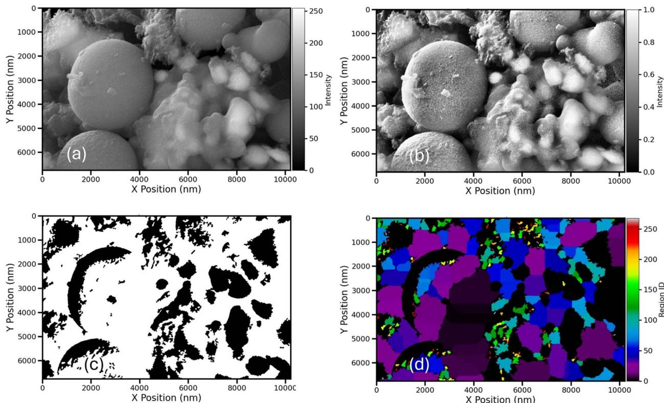
Fig. 16 SEM image analysis of the  $\text{Fe}_3\text{O}_4@PyTh$  nanocomposite. The X and Y axes are scaled in nanometers (nm). (a) Original region of interest (ROI); (b) high contrast processed ROI; (c) crystallite mask following segmentation; (d) labeled crystallites using watershed segmentation.
