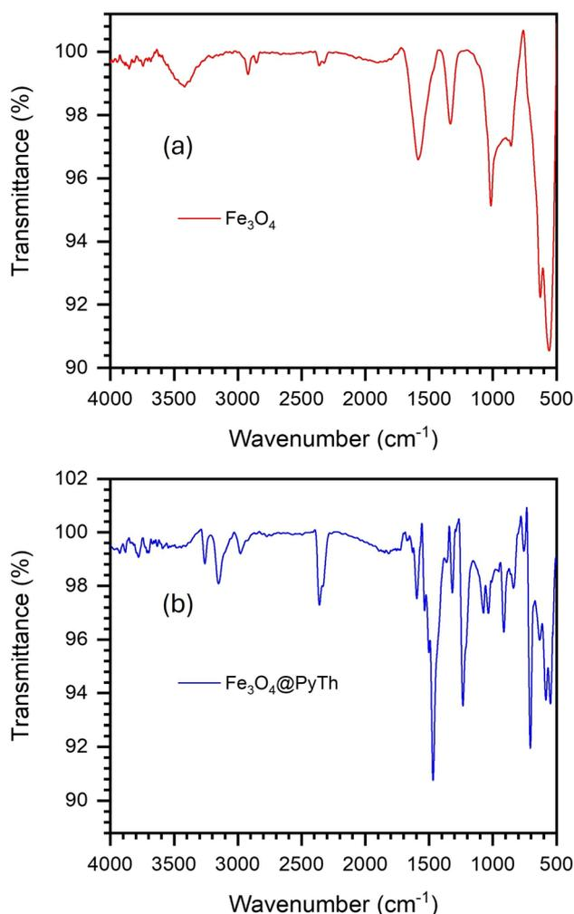
Fig. 5 FTIR characterization of  $\text{Fe}_3\text{O}_4$  nanoparticles and the  $\text{Fe}_3\text{O}_4@\text{PyTh}$  nanocomposite. (a) FTIR spectrum of pristine  $\text{Fe}_3\text{O}_4$  nanoparticles; (b) FTIR spectrum of the  $\text{Fe}_3\text{O}_4@\text{PyTh}$  nanocomposite.
