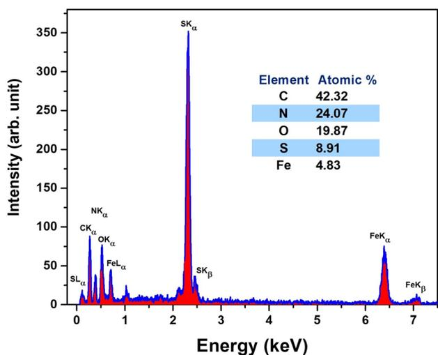
Fig. 13 EDX spectrum of the  $\text{Fe}_3\text{O}_4$ @PyTh nanocomposite, showing elemental peaks for Fe, O, C, N, and S. The inset table lists the atomic percentages of the detected elements, confirming successful surface functionalization with the pyrazolone–thiophene (PyTh) Schiff base.
