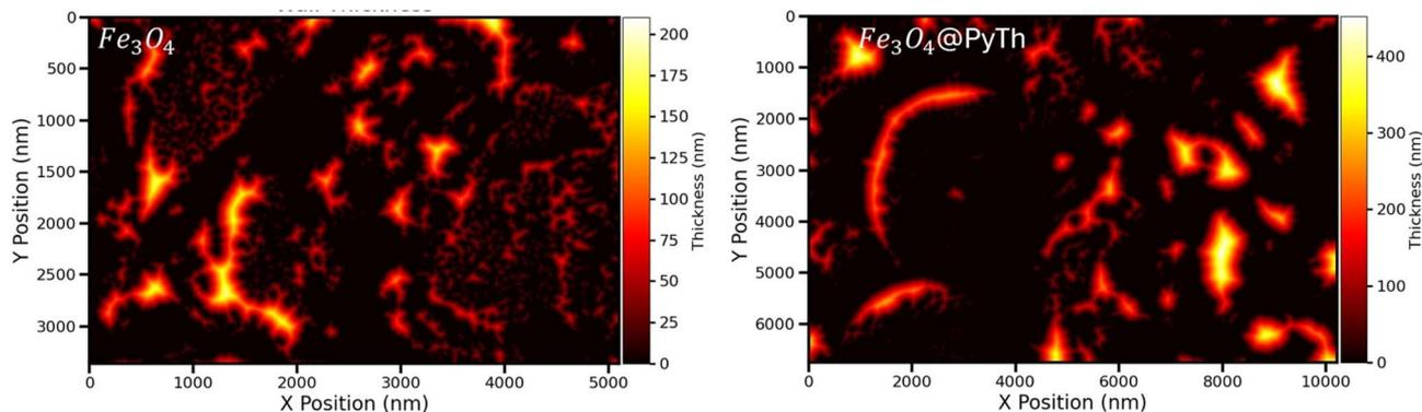
Fig. 18 Comparative wall thickness maps of  $\text{Fe}_3\text{O}_4$  (left) and  $\text{Fe}_3\text{O}_4@PyTh$  (right). The X and Y axes are scaled in nanometers (nm). Maps show local wall thickness (in nm) derived from SEM segmentation, with colour scales indicating the thickness magnitude.  $\text{Fe}_3\text{O}_4$  has thinner, highly connected walls, while  $\text{Fe}_3\text{O}_4@PyTh$  displays significant wall thickening after PyTh functionalization.
