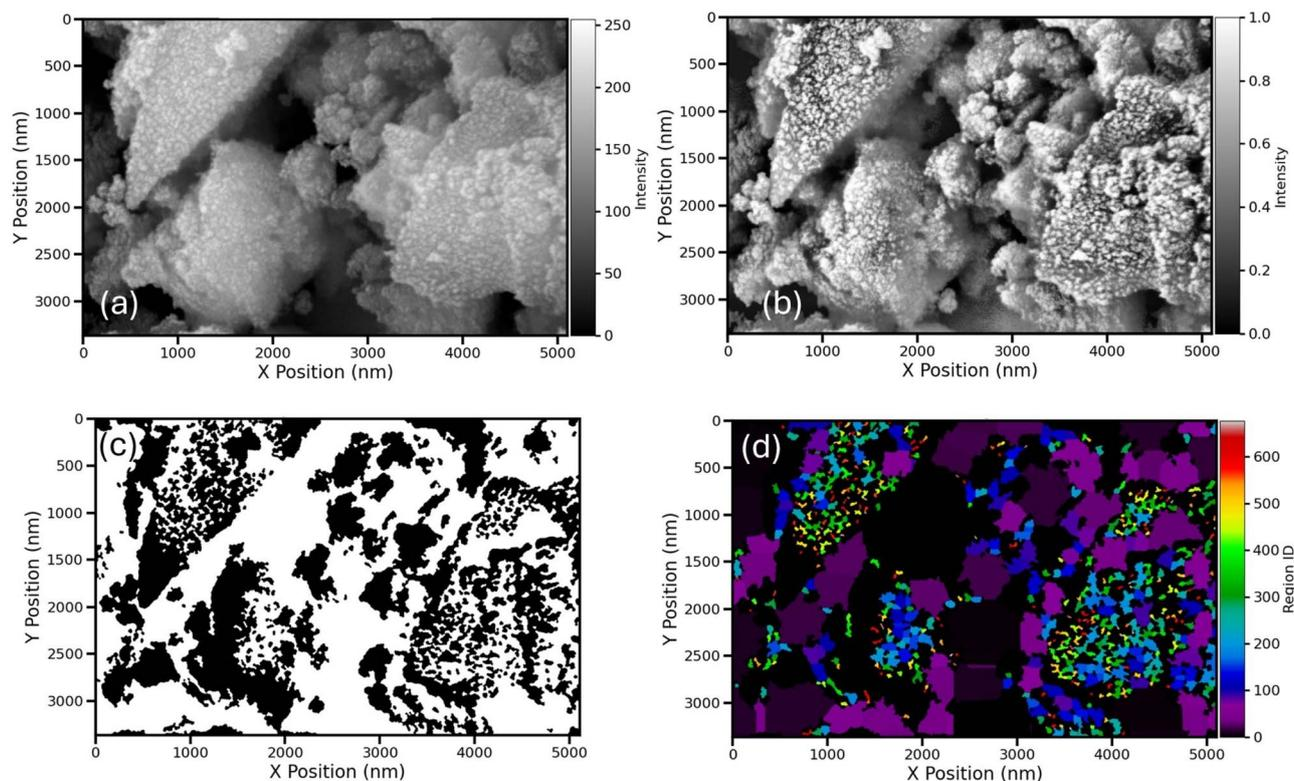
Fig. 14 SEM image analysis workflow for  $\text{Fe}_3\text{O}_4$  nanoparticles. The X and Y axes are scaled in nanometers (nm). (a) Original ROI showing densely packed nanoparticle clusters; (b) contrast-enhanced image highlighting crystallite boundaries and interparticle voids; (c) binary crystallite mask generated *via* *K*-means clustering and morphological filtering; (d) labelled crystallites segmented using watershed transformation, with unique colour coding for individual particles.
