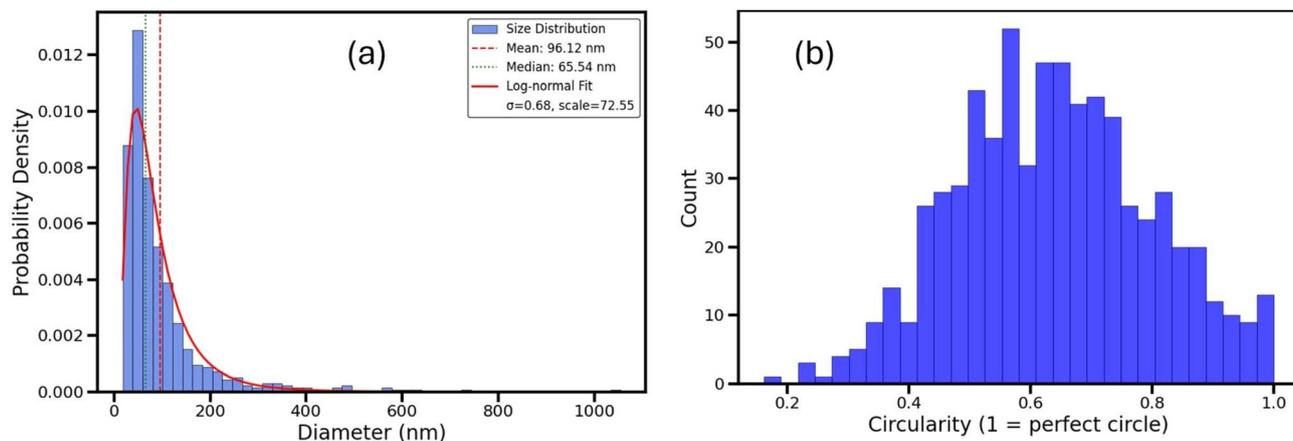
Fig. 15 Statistical analysis of  $\text{Fe}_3\text{O}_4$  crystallites from SEM images. (a) Crystallite size distribution with a log-normal fit (red line); (b) distribution of crystallite circularity, showing particle shape variation.
