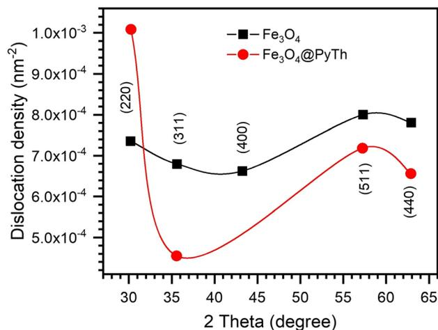
Fig. 12 Dislocation density vs.  $2\theta$  for  $\text{Fe}_3\text{O}_4$  and  $\text{Fe}_3\text{O}_4$ @PyTh, revealing comparable defect densities.
