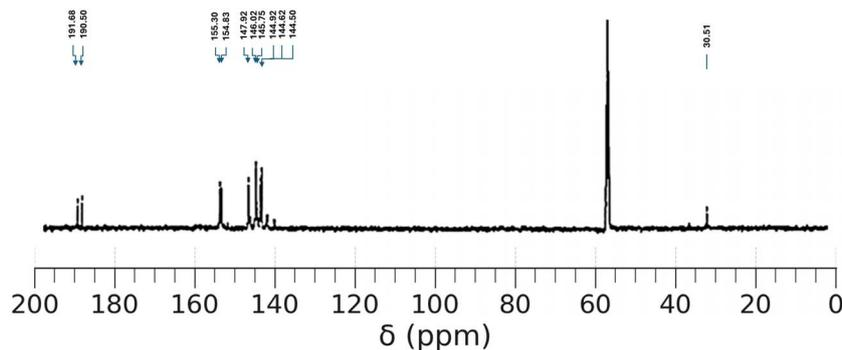
Fig. 2  $^{13}\text{C}$  NMR spectrum of the pyrazolone–thiophene Schiff base (PyTh), displaying characteristic carbon resonances that confirm the molecular architecture.
