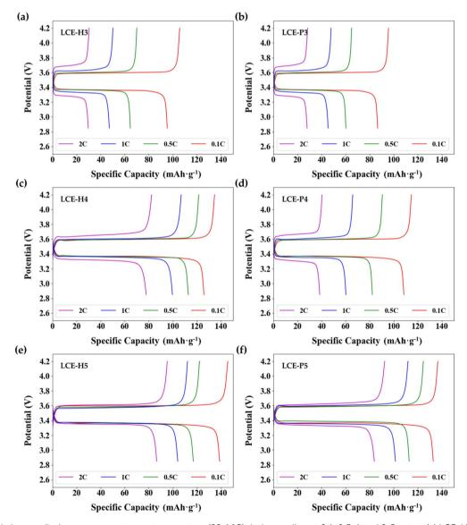
Fig. 10 Selected charge-discharge curves at room temperature (22.4 °C) during cycling at 0.1, 0.5, 1 and 2 C-rates: (a) LCE-H3, (b) LCE-P3, (c) LCE-H4, (d) LCE-P4, (e) LCE-H5, (f) LCE-P5.
