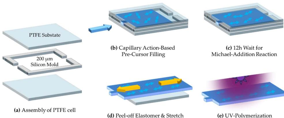
Fig. 2 Schematic illustration of the fabrication process for planar-aligned liquid crystal elastomer electrolytes (LCE-Pr). (a) Illustration of polytetrafluoroethylene (PTFE) sandwich cell mold used for precursor injection and alignment; (b–e) steps of the alignment and curing process. Alignment direction shown by yellow arrows.
