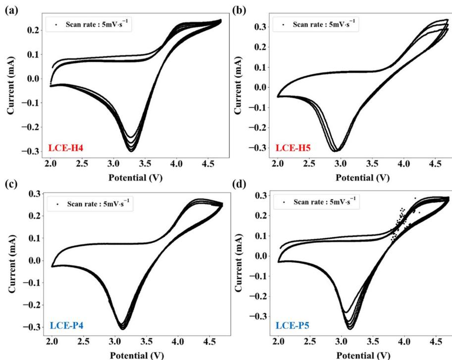
Fig. 8 Cyclic voltammograms recorded at  $5 \text{ mV s}^{-1}$  scan rate for (a) Li/LCE-H4/LiFePO<sub>4</sub>, (b) Li/LCE-H5/LiFePO<sub>4</sub>, (c) Li/LCE-P4/LiFePO<sub>4</sub>, and (d) Li/LCE-P5/LiFePO<sub>4</sub> cells.
