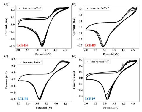
Fig. 8 Cyclic voltammograms recorded at 5 mV s<sup>-1</sup> scan rate for (a) Li/LCE-H4/LiFePO<sub>4</sub>, (b) Li/LCE-H5/LiFePO<sub>4</sub>, (c) Li/LCE-P4/LiFePO<sub>4</sub>, and (d) Li/LCE-P5/LiFePO₄ cells
