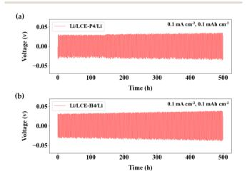
Fig. 7 Voltage profiles of symmetric Li/LCE-X4/Li cells at  $0.1 \, \text{mA cm}^{-2}$  current density and  $0.1 \, \text{mAh cm}^{-2}$  cycling capacity. (a) Planar alignment; (b) homeotropic alignment.
