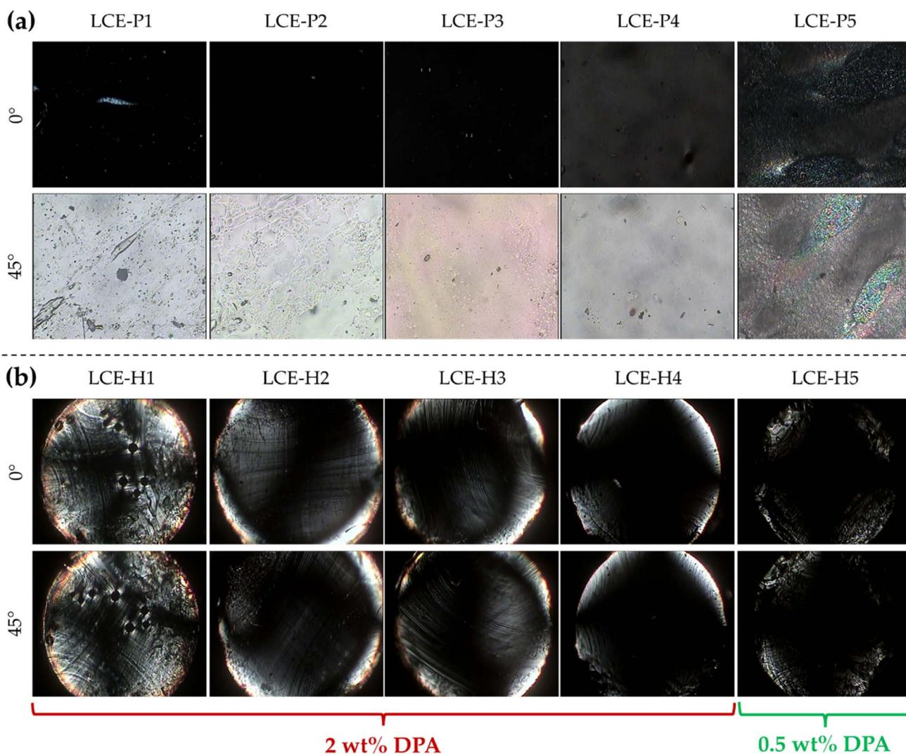
Fig. 5 POM textures of  $100 \text{ }\mu\text{m}$  thick LCE- $X_n$  ( $n = 1, 2, 3, 4, 5$ ) electrolytes observed under crossed polarizers at rotation angles of  $0^\circ$  and  $45^\circ$  with respect to the crossed polarizers for: (a) planar-aligned (LCE- $P_n$ ) and (b) homeotropically-aligned (LCE- $H_n$ ) samples. The DPA concentration used for each electrolyte's preparation is indicated below its respective POM images.
