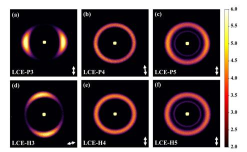
Fig. 15 2D Wide Angle X-ray (WAXS) profiles of LCE-Xn (n = 3-5) after 300 charge-discharge cycles. (a), (b) and (c) show results for LCP-P3,4 and 5, and (d), (e) and (f) show 2D profiles for LCP-H3,4 and 5, respectively. White double-sided arrows indicate the original alignment directions. Exposure time is 5 minutes for all samples.
