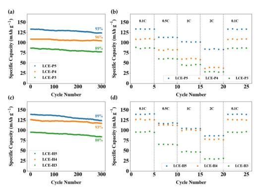
Fig. 11 Specific discharge capacity of Li/LCE-Xn/LiFePO<sub>4</sub> (n=3,4,5) during 300 cycles at 0.1C and room temperature: (a) planar alignment, (c) homeotropic alignment Rate performance of Li/LCE-Xn/LiFePO<sub>4</sub> (n=3,4,5) batteries at various C-rates at room temperature: (b) planar alignment, (d) homeotropic alignment.
