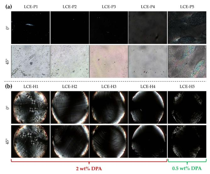
Fig. 5 POM textures of  $100 \mu m$  thick LCE-Xn (n = 1, 2, 3, 4, 5) electrolytes observed under crossed polarizers at rotation angles of  $0^{\circ}$  and  $45^{\circ}$  with respect to the crossed polarizers for: (a) planar-aligned (LCE-Pn) and (b) homeotropically-aligned (LCE-Hn) samples. The DPA concentration used for each electrolyte's preparation is indicated below its respective POM images.
