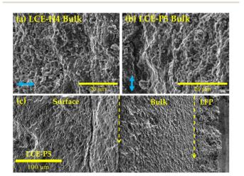
Fig. 13 SEM images of electrolytes after 300 charge–discharge cycles showing cross-sectional views of the bulk material for (a) LCE-H4; (b) LCE-P5; and (c) 45° tilt angle view of LCE-P5 electrolyte anode-side surface, bulk and LFP cathode. Blue arrows indicate the nematic director of the elastomer.
