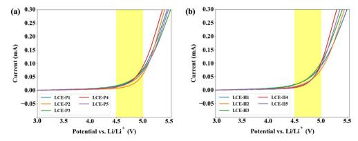
Fig. 9 Linear Sweep Voltammetry (LSV) of Li/LCE-Xn (n = 1, 2, 3, 4, 5) half cells showing the determination of the onset oxidation potential highlighted in the 4.5–5.0 V range and found to be  $\sim$ 4.8 V for (a) planar, and (b) homeotropic alignments.
