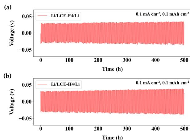
Fig. 7 Voltage profiles of symmetric  $\text{Li/LCE-X4/Li}$  cells at  $0.1 \text{ mA cm}^{-2}$  current density and  $0.1 \text{ mAh cm}^{-2}$  cycling capacity. (a) Planar alignment; (b) homeotropic alignment.
