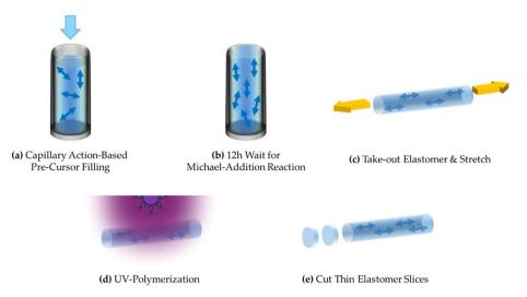
Fig. 3 Schematic illustration of the fabrication process for homeotropically aligned LCE electrolytes (LCE-Hn). (a—e) Steps of the alignment and curing process. Alignment direction shown by yellow arrows.
