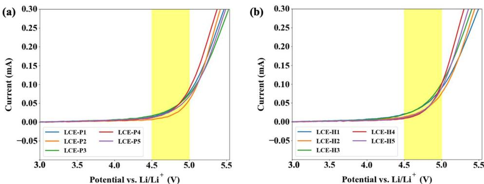
Fig. 9 Linear Sweep Voltammetry (LSV) of Li/LCE-X $n$  ( $n = 1, 2, 3, 4, 5$ ) half cells showing the determination of the onset oxidation potential highlighted in the  $4.5-5.0 \text{ V}$  range and found to be  $\sim 4.8 \text{ V}$  for (a) planar, and (b) homeotropic alignments.
