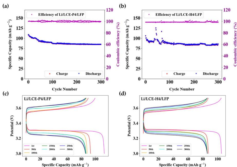
Fig. 12 Cycling performance of Li/LCE- $X_4$ /LiFePO<sub>4</sub> cells at 1C at room temperature. Cycle number dependence of specific capacity (left axis) and coulombic efficiency (right axis) for planar (a) and homeotropic alignment (b). Potential versus specific capacity (charge-discharge profiles) for planar (c) and homeotropic (d) alignment.
