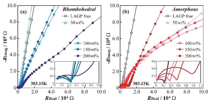
Fig. 5 Impedance spectra of [SUS/electrolyte/SUS] symmetric cells employing polyether-based hybrid electrolytes at 303.15 K: (a) rhombohedral LAGP and (b) amorphous LAGP.
