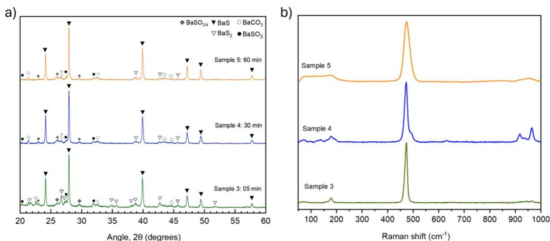
**Fig. 4** Time-dependent conversion kinetics at 500 °C. (a) XRD diffractograms of precursor powder (2 : 3 Ba(OH)<sub>2</sub> : S ratio) annealed at: 500 °C for 60 minutes (Sample 5, orange), 30 minutes (Sample 4, blue), and 05 minutes (Sample 3, green). (b) Corresponding Raman spectra demonstrating continuous decrease in BaS<sub>2</sub> signal intensity (474 cm<sup>-1</sup>) with extended dwell time, while BaS (Raman-inactive) increases.
