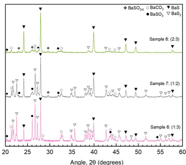
Fig. 5 XRD diffractograms of annealed samples (500 °C for 30 minutes) with varying quantities of sulfur: 2 mol  $\text{Ba}(\text{OH})_2$  per 3 mol sulfur (Sample 8, light green), 1 mol  $\text{Ba}(\text{OH})_2$  per 2 mol sulfur (Sample 7, grey), 1 mol  $\text{Ba}(\text{OH})_2$  per 3 mol sulfur (Sample 6, pink).
