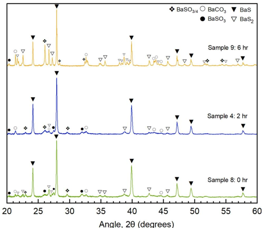
**Fig. 6** XRD diffractograms of precursor powder (2 : 3 Ba(OH)<sub>2</sub> : S ratio) annealed at 500 °C for 30 minutes after milling at 600 rpm for different durations: 6 hours milling (Sample 9, yellow), 2 hours milling (Sample 4, blue), 0 hours milling (Sample 8, light green).
