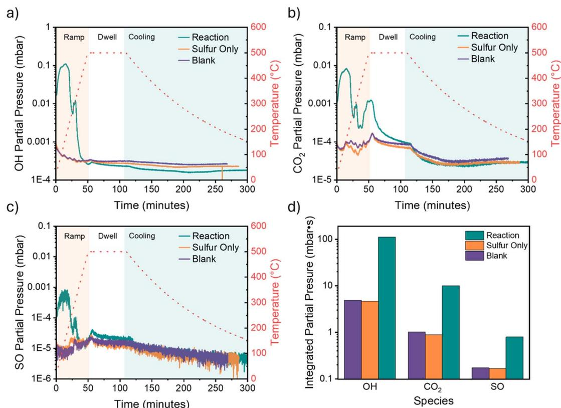
Fig. 7 The partial pressures measured during the furnace run of a reaction filled tube, sulfur only tube and empty tube (blank) monitoring (a) OH, (b) CO<sub>2</sub> and (c) SO. The integrated partial pressures over the full run are shown in (d).
