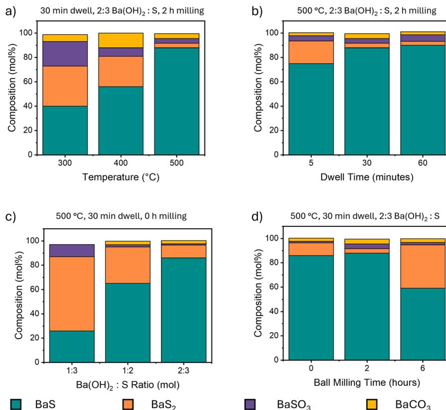
Fig. 2 Systematic optimisation of BaS synthesis conditions. Stacked bar charts showing phase composition (mol%) as a function of (a) annealing temperature, (b) dwell time at 500 °C, (c) Ba(OH)<sub>2</sub> : S ratio and (d) ball milling duration. Optimal conditions (500 °C, 30–60 minutes, 2 : 3 Ba(OH)<sub>2</sub> : S ratio and 2 hours milling) yield 88–90% BaS with minimal impurities.
