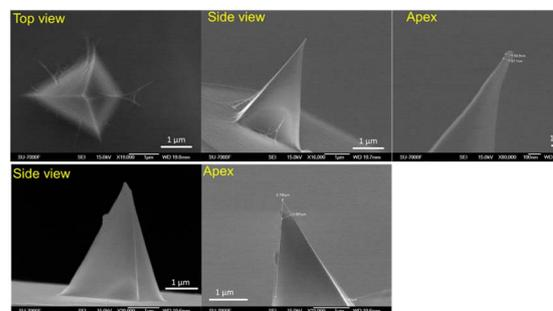
Fig. 1 Representative SEM images of the colloidal probes: (upper panel) top, side, and apex views of the HCNF-modified colloidal probe; (bottom panel) side and apex views of a used unmodified (naked) probe.
