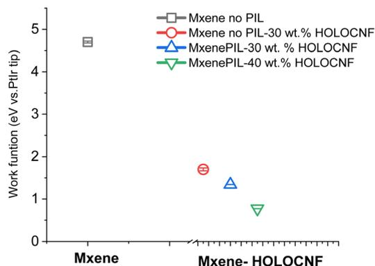
Fig. 4 Statistical analysis of the surface potentials for Mxene and the three types of MXene-HCNF composites, (note: KPFM results are reused from our abstract).<sup>22</sup>
