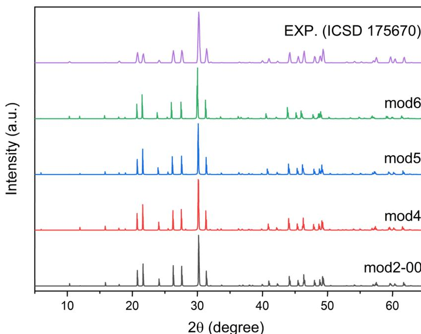
Fig. 3 Simulated XRD patterns for mod2-00, mod4, mod5, mod6 and the experimentally reported XRD pattern for  $\text{Pb}_{7.629}\text{Cu}_{2.371}(\text{PO}_4)_6\text{O}$  from ICSD.
