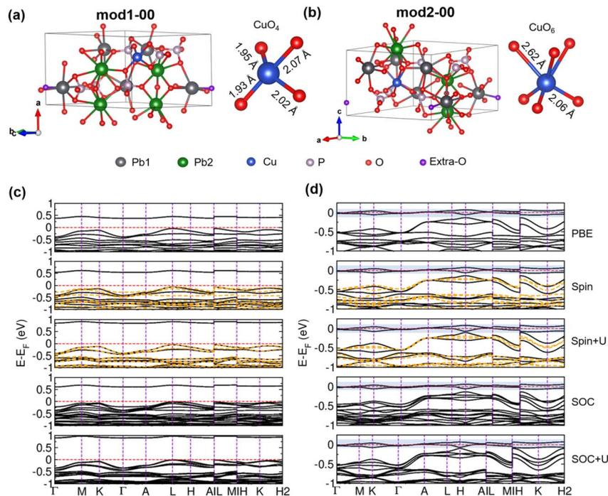
Fig. 4 (a) Crystal structure of the mod1-00 configuration, highlighting the Cu-centered O coordination environment ( $\text{CuO}_4$  polyhedron). (b) Crystal structure of mod2-00, featuring the corresponding  $\text{CuO}_6$  polyhedron. (c) Band structure of mod1-00 and (d) mod2-00 at five different levels: standard PBE (non-spin-polarized), spin-polarized PBE, spin-polarized PBE+ $U$ , SOC, and SOC+ $U$ .
