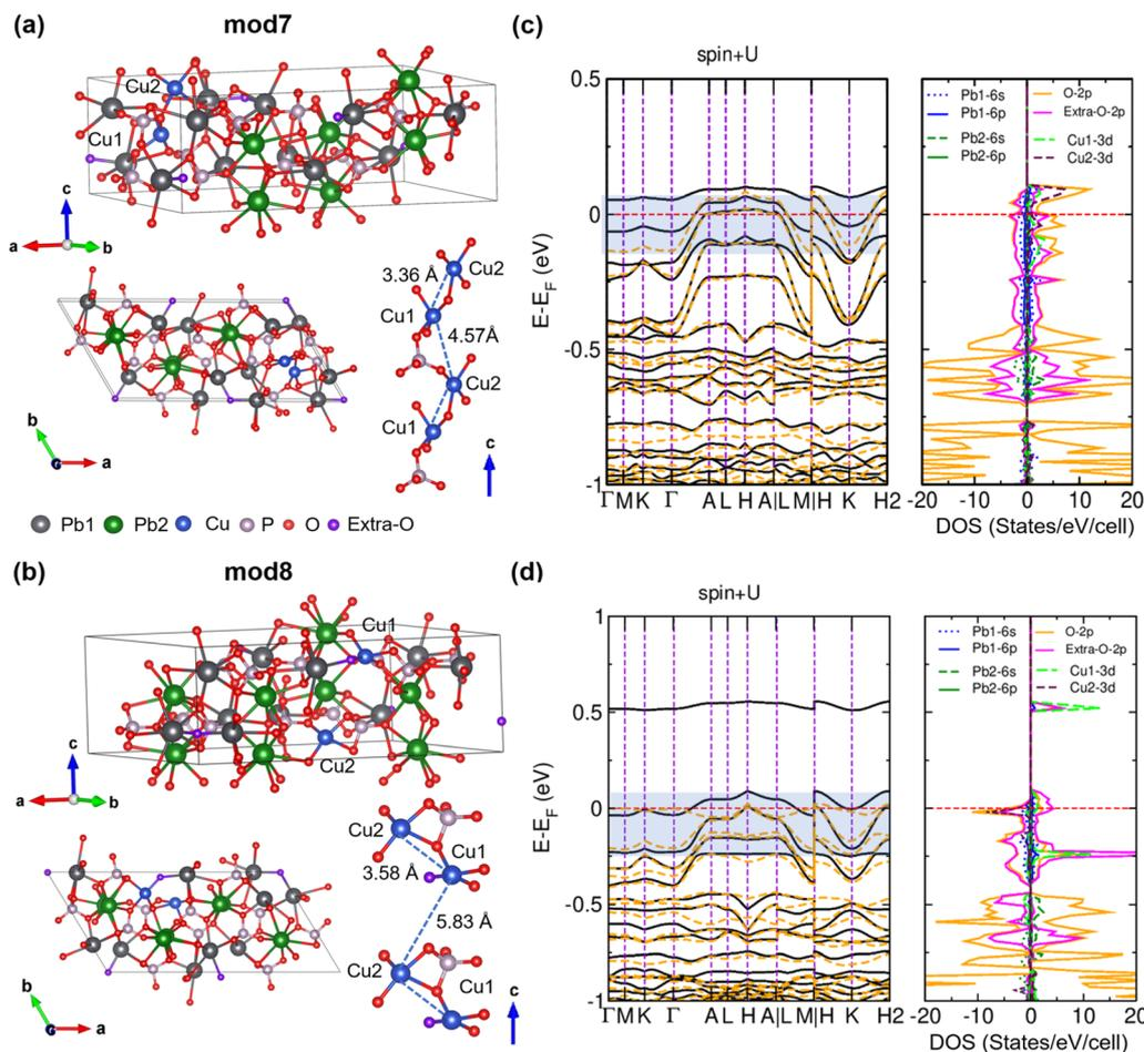
Fig. 8 (a and b) Crystal structures of mod7 and mod8, respectively, both exhibiting one-dimensional zig-zag Cu–Cu chains along the *c*-axis. (c and d) Corresponding band structures and PDOS for mod7 and mod8, respectively.
