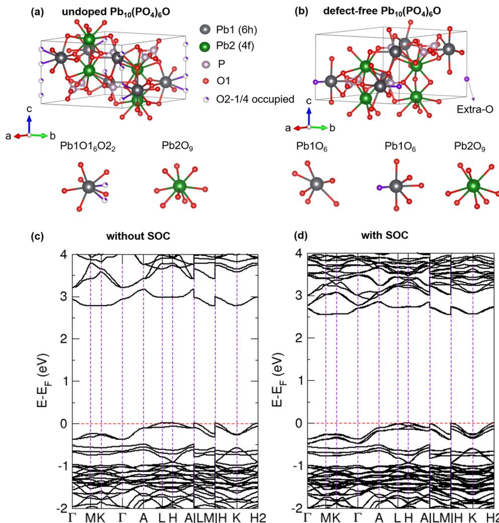
**Fig. 1** (a) Crystal structure of experimental  $\text{Pb}_{10}(\text{PO}_4)_6\text{O}$ , illustrating the coordination polyhedron of  $\text{Pb1O}_6\text{O}_{22}$  and  $\text{Pb2O}_9$ . (b) Crystal structure of defect-free  $\text{Pb}_{10}(\text{PO}_4)_6\text{O}$  model, showing the  $\text{Pb1O}_6$  and  $\text{Pb2O}_9$  coordination polyhedrons. (c) and (d) Band structure of defect-free  $\text{Pb}_{10}(\text{PO}_4)_6\text{O}$  model (c) without and (d) with SOC effect.
