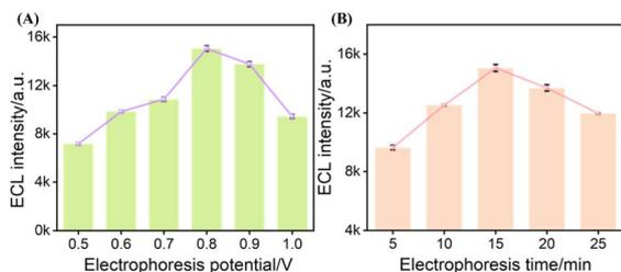
Fig. 8 ECL responses of NGQDs@NH<sub>2</sub>-VMSF/ITO electrodes prepared at different electrophoretic potentials (A) and electrophoresis times (B).
