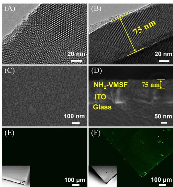
Fig. 4 (A and B) TEM images of the surface (A) and cross-section (B) of the NH<sub>2</sub>-VMSF. (C and D) SEM images of the surface (C) and cross-section (D) of the NH<sub>2</sub>-VMSF/ITO electrode. (E and F) Confocal laser microscopy images of NH<sub>2</sub>-VMSF/ITO (E) and NGQDs@NH<sub>2</sub>-VMSF/ITO (F). The insets show the corresponding bright-field images. Excitation wavelength: 488 nm.
