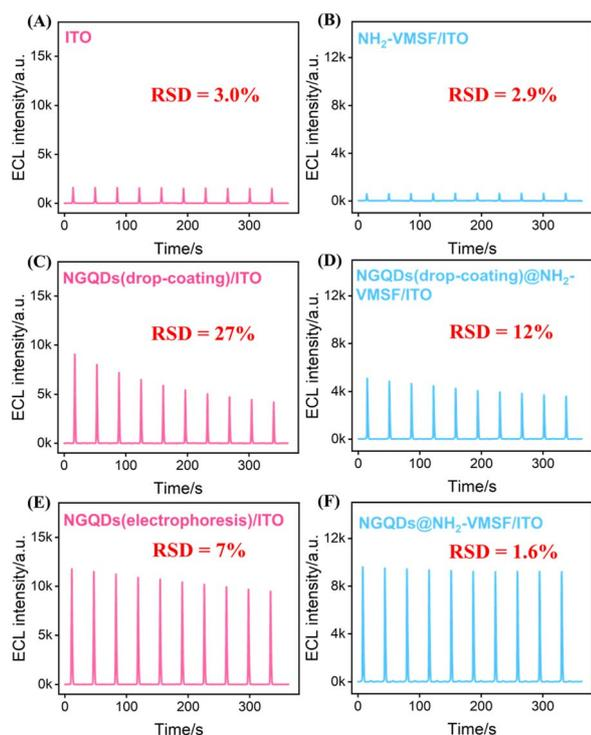
Fig. 6 ECL intensity–time curves obtained at (A) ITO, (B) NH<sub>2</sub>-VMSF/ITO, (C) NGQDs(drop-coating)/ITO, (D) NGQDs(drop-coating)@NH<sub>2</sub>-VMSF/ITO, (E) NGQDs(electrophoresis)/ITO, and (F) NGQDs@NH<sub>2</sub>-VMSF/ITO electrodes. The PMT voltage was set at 600 V.
