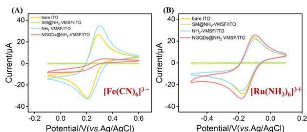
Fig. 5 CV curves of bare ITO, SM@NH<sub>2</sub>-VMSF/ITO, NH<sub>2</sub>-VMSF/ITO and NGQDs@NH<sub>2</sub>-VMSF/ITO in (A) [Fe(CN)<sub>6</sub>]<sup>3-</sup> or (B) [Ru(NH<sub>3</sub>)<sub>6</sub>]<sup>3+</sup> solutions. The redox concentration was 0.5 mM and the electrolyte was 0.05 M KHP solution. Scan rate in CV measurement was 50 mV s<sup>-1</sup>.
