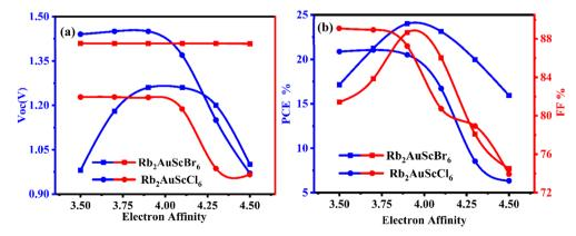
Fig. 11 Effect of absorber electron affinity on performance parameters (a)  $V_{\rm oc}$  and  $J_{\rm sc}$ , (b) PCE and FF of (ITO/IGZO/Rb<sub>2</sub>AuScBr<sub>6</sub>/CBTS/Ni) (ITO/WS<sub>2</sub>/Rb<sub>2</sub>AuScCl<sub>6</sub>/CBTS/Ni) devices.
