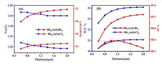
Fig. 7 Effect of absorber thickness on performance parameters (a)  $V_{\rm oc}$ , and  $J_{\rm sc}$ , (b) PCE and FF of (ITO/IGZO/Rb<sub>2</sub>AuScBr<sub>6</sub>/CBTS/Ni) (ITO/WS<sub>2</sub>/Rb<sub>2</sub>AuScCl<sub>6</sub>/CBTS/Ni) devices.
