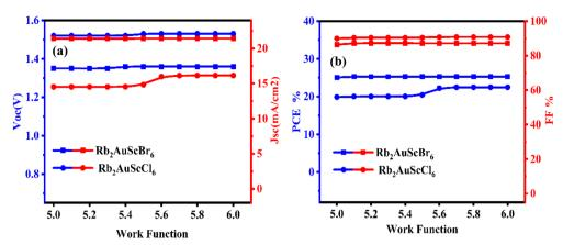
Fig. 8 Effect of Metal Back Contact on performance parameters (a)  $V_{\rm oc}$ , and  $J_{\rm sc}$ , (b) PCE and FF of (ITO/IGZO/Rb<sub>2</sub>AuScBr<sub>6</sub>/CBTS/Ni) (ITO/WS<sub>2</sub>/Rb<sub>2</sub>AuScCl<sub>6</sub>/CBTS/Ni) devices.
