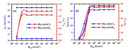
Fig. 14 Effect of shunt resistance ( $R_{sh}$ ) on performance parameters (a)  $V_{oc}$  and  $J_{sc}$ , (b) PCE and FF of (ITO/IGZO/Rb<sub>2</sub>AuScBr<sub>6</sub>/CBTS/Ni) (ITO/WS<sub>2</sub>/Rb<sub>2</sub>AuScCl<sub>6</sub>/CBTS/Ni) devices.
