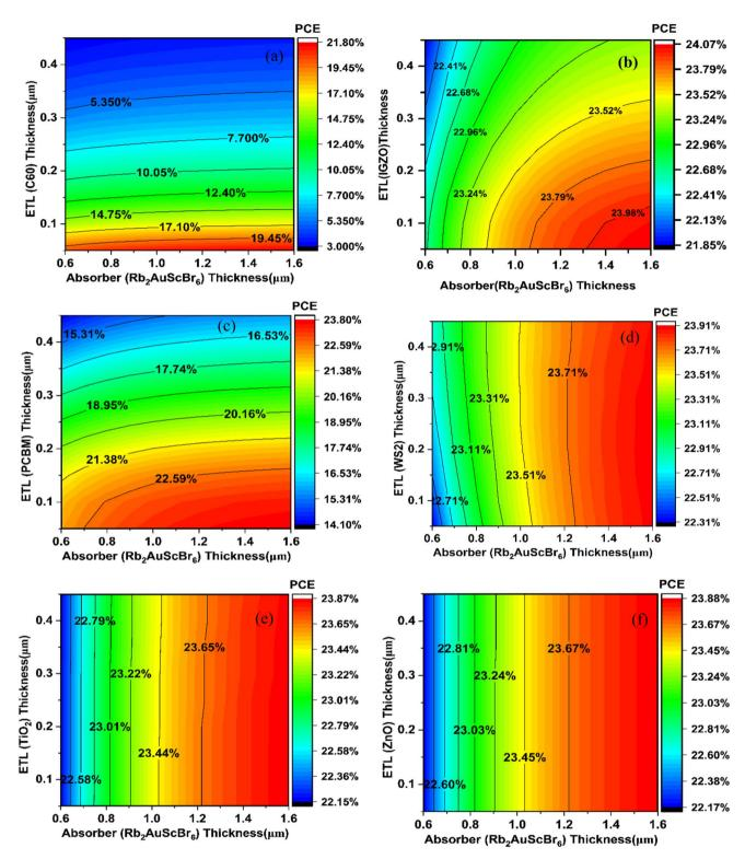
Fig. 5 Contour mapping of PCE, when the absorber is  $Rb_2AuScBr_6$  and ETLs as (a)  $C_{60}$ . (b) IGZO, (c) PCBM, (d) WS<sub>2</sub>, (e) TiO<sub>2</sub> and (f) ZnO.
