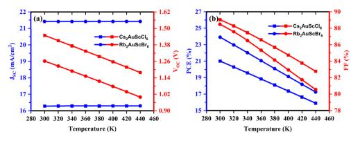
Fig. 15 Effect of temperature on performance parameters (a)  $V_{\rm oc}$  and  $J_{\rm sc}$ , (b) PCE and FF of (ITO/IGZO/Rb<sub>2</sub>AuScBr<sub>6</sub>/CBTS/Ni) and (ITO/WS<sub>2</sub>/Rb<sub>2</sub>AuScCl<sub>6</sub>/CBTS/Ni) devices.
