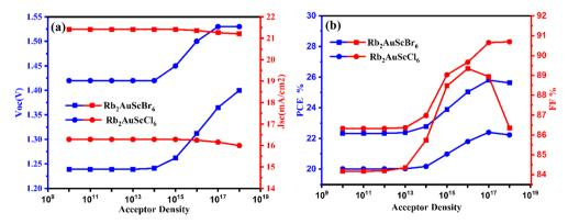
Fig. 9 Variation of cell parameters with changing acceptor density (a)  $V_{oc}$  and  $J_{sc}$ , (b) PCE and FF of (ITO/IGZO/Rb<sub>2</sub>AuScBr<sub>6</sub>/CBTS/Ni) and (ITO/WS<sub>2</sub>/Rb<sub>2</sub>AuScCl<sub>6</sub>/CBTS/Ni) devices.
