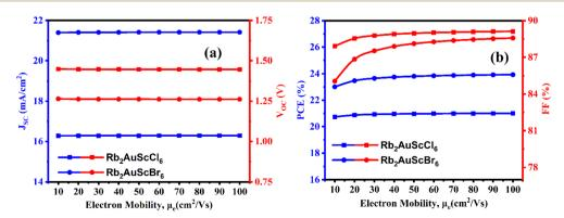
Fig. 12 Effect of absorber electron mobility on performance parameters (a)  $V_{oc}$  and  $J_{sc}$ , (b) PCE and FF of (ITO/IGZO/Rb<sub>2</sub>AuScBr<sub>6</sub>/CBTS/Ni) (ITO/IGZO/Rb<sub>2</sub>AuScBr<sub>6</sub>/CBTS/Ni) (ITO/IGZO/Rb<sub>2</sub>AuScBr<sub>6</sub>/CBTS/Ni) WS2/Rb2AuScCl6/CBTS/Ni) devices
