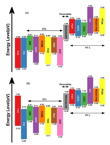
Fig. 2 Energy band alignment between the different ETL and HTL materials of (a) Rb<sub>2</sub>AuScBr<sub>6</sub> absorber and (b) Rb<sub>2</sub>AuScCl<sub>6</sub> absorber.
