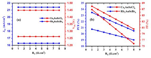
Fig. 13 Effect of series resistance ( $R_s$ ) on performance parameters (a)  $V_{oc}$  and  $J_{sc}$ , (b) PCE and FF of (ITO/IGZO/Rb<sub>2</sub>AuScBr<sub>6</sub>/CBTS/Ni) (ITO/WS<sub>2</sub>/Rb<sub>2</sub>AuScCl<sub>6</sub>/CBTS/Ni) devices.
