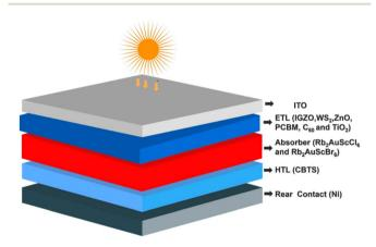
Fig. 1 The design configuration of the Rb<sub>2</sub>AuScCl<sub>6</sub> and Rb<sub>2</sub>AuScBr<sub>6</sub>: based PSC.
