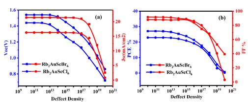
Fig. 10 Effect of absorber defect density ( $N_t$ ) on performance parameters (a)  $V_{oc}$  and  $J_{sc}$ , (b) PCE and FF of (ITO/IGZO/Rb<sub>2</sub>AuScBr<sub>6</sub>/CBTS/Ni) (ITO/WS<sub>2</sub>/Rb<sub>2</sub>AuScCl<sub>6</sub>/CBTS/Ni) devices.
