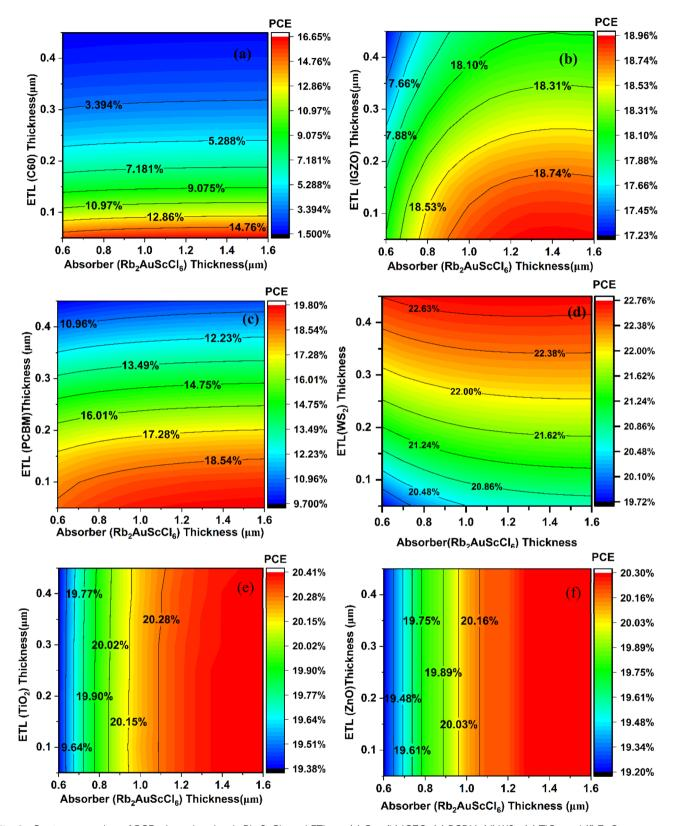
Fig. 6 Contour mapping of PCE when absorber is  $Rb_2ScCl_6$  and ETLs as (a)  $C_{60}$ , (b) IGZO, (c) PCBM, (d) WS<sub>2</sub>, (e) TiO<sub>2</sub> and (f) ZnO<sub>2</sub>
