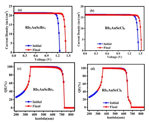
Fig. 17 (a and b) J-V characteristics and (c and d) QE curve of Rb<sub>2</sub>AuScBr<sub>6</sub> and Rb<sub>2</sub>AuScCl<sub>6</sub>-baesd absorber initial and final devices.
