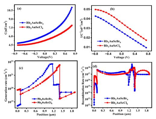
Fig. 16 (a) Capacitance, (b) Mott–Scotty plot  $(1/C^2)$ , (c) generation, and (d) recombination of (ITO/IGZO/Rb<sub>2</sub>AuScBr<sub>6</sub>/CBTS/Ni) and (ITO/WS<sub>2</sub>/Rb<sub>2</sub>AuScCl<sub>6</sub>/CBTS/Ni) devices.
