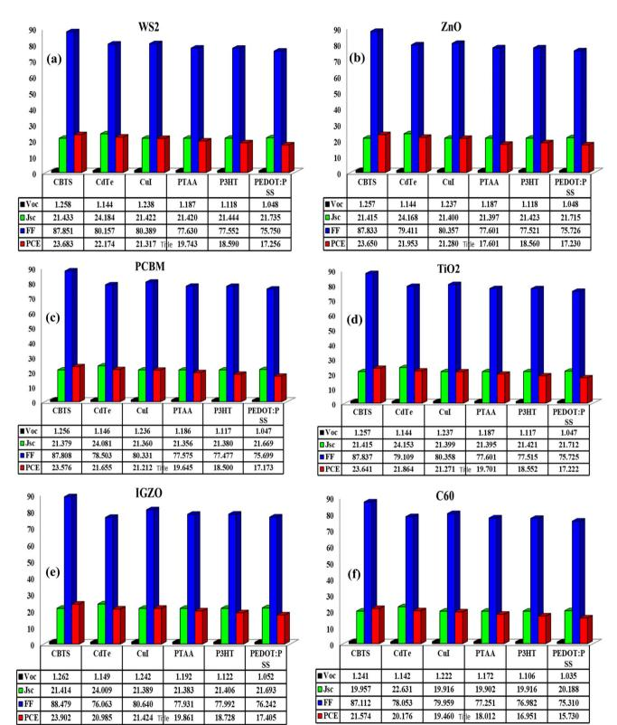
Fig. 3 HTL & ETL selection for Rb<sub>2</sub>AuScBr<sub>6</sub> of (a) WS<sub>2</sub> (b) ZnO (c) PCBM, (d) TiO<sub>2</sub>, (e) IGZO and (f) C<sub>60</sub> with HTL of CBTS, CdTe, CuI, PTAA, P3HT and PEDOT: PSS.
