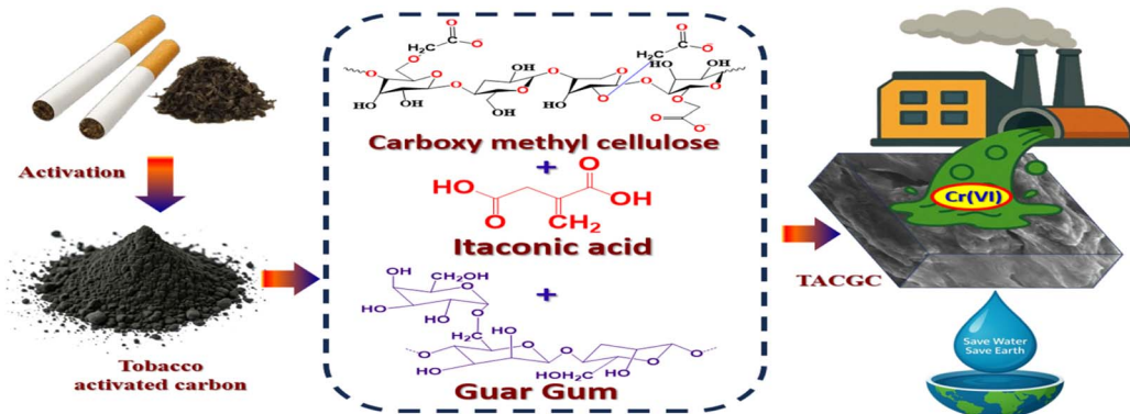
Fig. 1 Representation illustration of synthesis of TACGC composite sponge.
