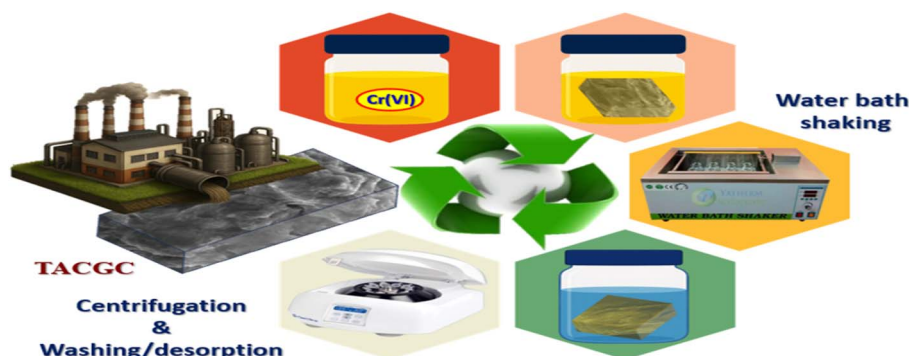
Fig. 2 Diagrammatic representation of Cr(vi) adsorption and elimination onto TACGC.
