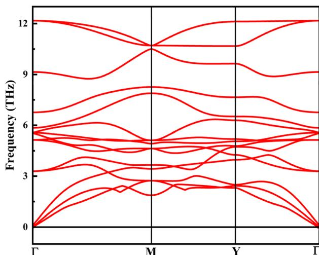
Fig. 2 Phonon dispersion curve for  $\text{Cr}_2\text{S}_2\text{Se}$  monolayer.
