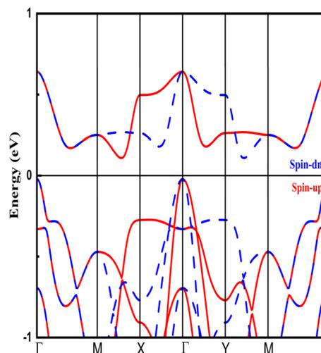
Fig. 4 The obtained band structure for  $\text{Cr}_2\text{S}_2\text{Se}$  monolayer.
