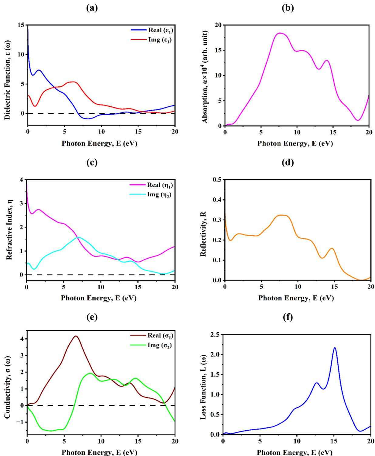
Fig. 3 The optical response of Sr<sub>3</sub>BiI<sub>3</sub> anti-perovskite was systematically analyzed through its (a) dielectric function, (b) absorption behavior, (c) refractive index, (d) reflectivity, (e) optical conductivity, and (f) electron energy loss spectrum.
