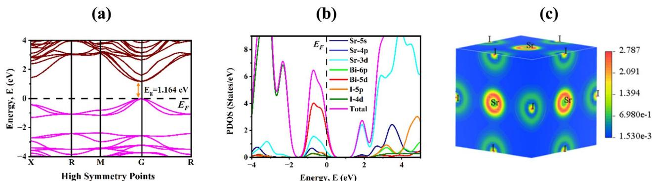
Fig. 2 Electronic properties of  $\text{Sr}_3\text{BiI}_3$  anti-perovskite showing (a) band gap, (b) DOS, and (c) charge density distribution.
