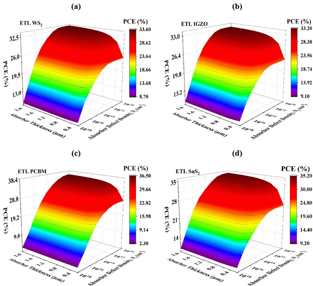
Fig. 10 Examining the impact of  $N_t$  and  $\text{Sr}_3\text{Bi}_2\text{I}_3$  thickness on PCE in various ETL configurations: (a)  $\text{WS}_2$ , (b) IGZO, (c) PCBM, and (d)  $\text{SnS}_2$ .
