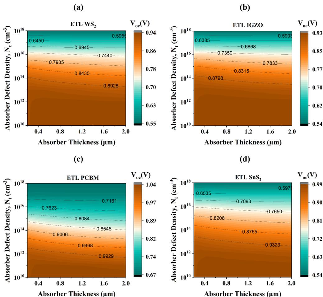
Fig. 7 Examining the impact of  $N_t$  and  $\text{Sr}_3\text{BiI}_3$  thickness on  $V_{OC}$  in various ETL configurations: (a)  $\text{WS}_2$ , (b) IGZO, (c) PCBM, and (d)  $\text{SnS}_2$ .
