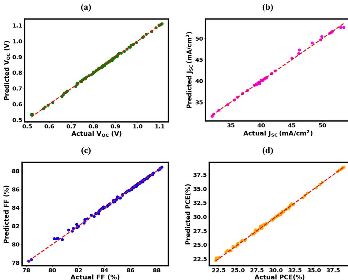
Fig. 18 Al/FTO/SnS<sub>2</sub>/Sr<sub>3</sub>BiI<sub>3</sub>/CBTS/Ni cell performance evaluation: a ML comparison of predicted and actual results for (a)  $V_{OC}$ , (b)  $J_{SC}$ , (c) FF, and (d) PCE.
