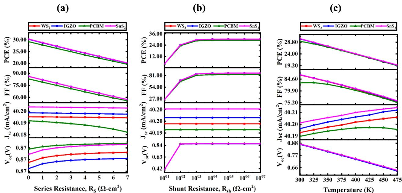
Fig. 14 Impact of (a) series, (b) shunt resistance, and (c) temperature on performance metrics.
