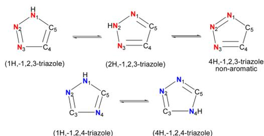
Fig. 1 Isomeric structures of 1,2,3- and 1,2,4-triazoles.
