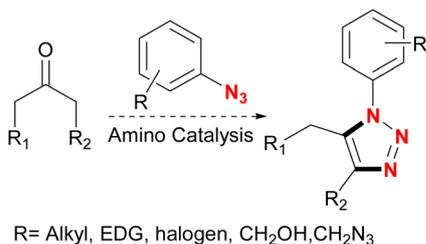
Scheme 26 Synthesis of 1,2,3-triazoles from unactivated ketones.
