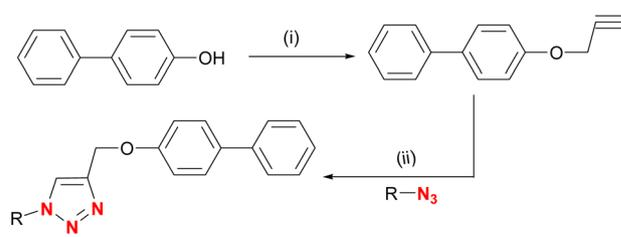
Scheme 12 Synthesis of 1,2,3-triazoles from *p*-hydroxy diphenyl and propargyl bromide. (i) Propargyl bromide,  $\text{K}_2\text{CO}_3$ , DMF, 90%; (ii) CuI (1 mol%), DHQD<sub>2</sub>(PHAL) (1 mol%),  $\text{H}_2\text{O}/\text{DCM}$  (1 : 1), RT, 0.5–2 h, 80–96%.
