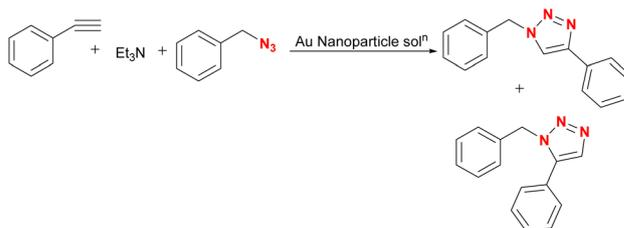
Scheme 61 Synthesis of 1,2,3-triazoles using gold nanoparticles.
