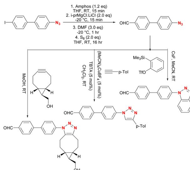
Scheme 21 Synthesis of triazoles *via* organo-magnesium intermediates.
