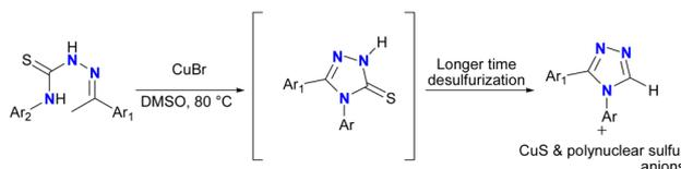
**Scheme 36** Synthesis of 1,2,4-triazoles *via* C–N bond formation.
