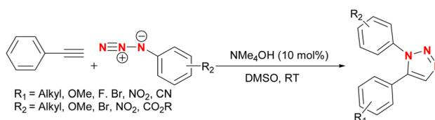
Scheme 25 Synthesis of 1,2,3-triazoles *via* azide-alkyne cycloaddition.
