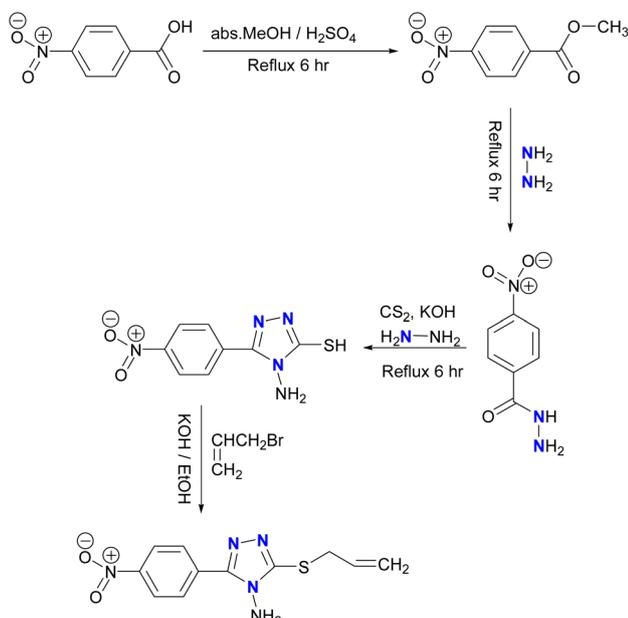
Scheme 50 Synthesis of 1,2,4-triazoles from 3-(4-nitrobenzoyl) dithiocarbazate.
