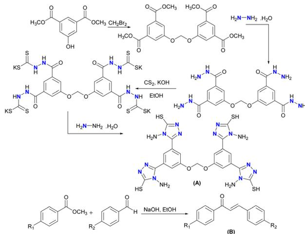
Scheme 55 Synthesis of 1,2,4-triazoles from dimethyl-4-hydroxyisophthalate and dibromomethane.
