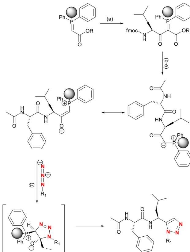
Scheme 24 Synthesis of peptide derivatives of 1,2,3-triazoles. (a) Fmoc-Leu-OH and MSNT, lutidine in CH<sub>2</sub>Cl<sub>2</sub> or BTFFH, DIPEA, DMF (R = TMSE or tertbutyl), 14 h; (b) 20% piperidine/DMF; (c) Fmoc-Phe-OH, DIC, HOBT, DMF, 2 h; (d) 20% Ac<sub>2</sub>O/DMF or (e) TAS-F/DMF or TFA/CH<sub>2</sub>Cl<sub>2</sub> (R = TMSE or tertbutyl); and (f) 4–14, CH<sub>2</sub>Cl<sub>2</sub>, or THF.
