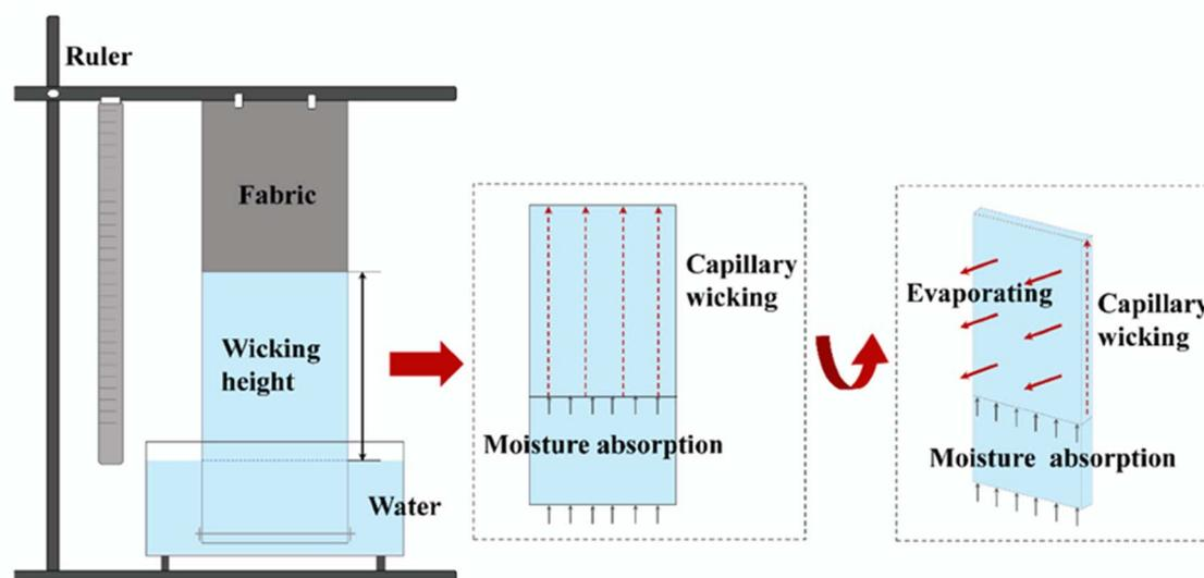
Fig. 5 Water wicking and evaporating occur simultaneously in a typical vertical wicking test. Published by the CC-BY license<sup>73</sup> Copyright 2020, The authors. Published by MDPI, Basel, Switzerland.
