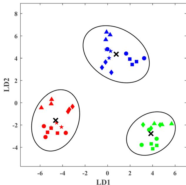
Fig. 8 LDA analysis for adulteration of milk with  $\text{H}_2\text{O}_2$  (green),  $\text{Cr}(\text{vi})$  (blue) and  $\text{ClO}^-$  (red). Level 1: ●, Level 2: ▲, Level 2: ★, Level 4: ■, Level 5: ◆. Details of concentration levels are provided in Fig. 7.
