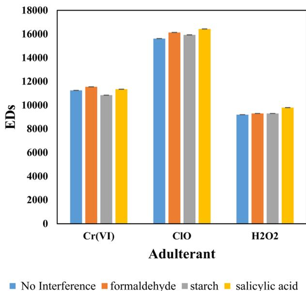
Fig. 11 Interference evaluation of proposed colorimetric sensor array for detection of  $\text{H}_2\text{O}_2$  (21.6  $\text{mmol L}^{-1}$ ),  $\text{ClO}^-$  (0.9  $\text{mmol L}^{-1}$ ),  $\text{Cr}(\text{VI})$  (0.34  $\text{mmol L}^{-1}$ ) in the presence of various adulterants with concentration of 10  $\text{mmol L}^{-1}$  and  $N = 3$ .
