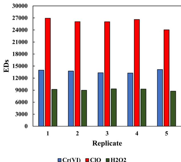
Fig. 5 The reproducibility of the response of sensor array for detection of milk adulterants (blue) 0.85 mmol L<sup>-1</sup> of Cr(vi), (red) 2.01 mmol L<sup>-1</sup> of ClO<sup>-</sup>, (green) 21.6 mmol L<sup>-1</sup> of H<sub>2</sub>O<sub>2</sub>.
