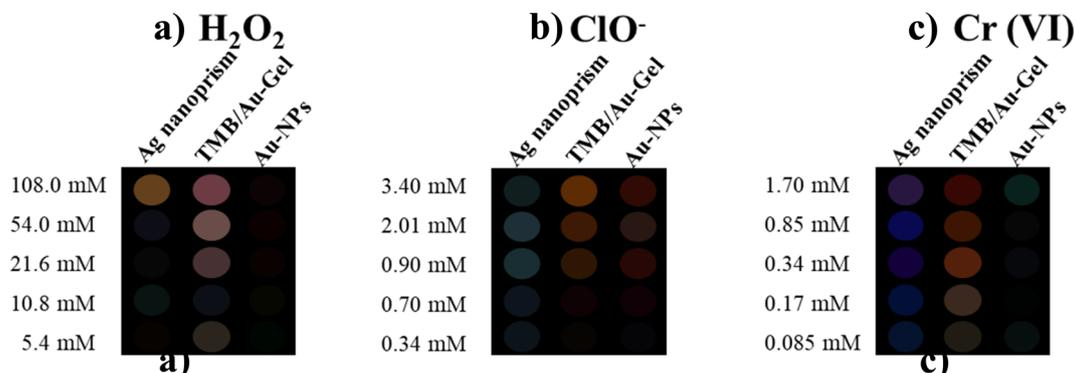
Fig. 6 Color-difference maps of studied milk adulterants (a) H<sub>2</sub>O<sub>2</sub>, (b) ClO<sup>-</sup>, (c) Cr(vi) at different concentration levels.
